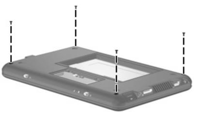
Where used: Four screws that secure the top cover to the base enclosure
