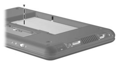
Where used: One screw that secures the keyboard to the device
