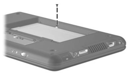
Where used: One screw that secures the keyboard to the device
