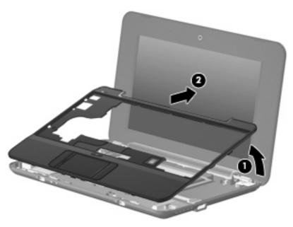
8. Release the ZIF connector (1) to which the TouchPad button board cable is connected, and then disconnect the cable (2) from the system board.
