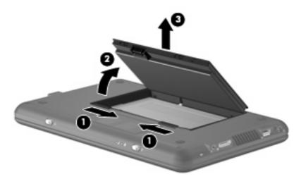
To install the battery, insert the rear edge of the battery into the battery bay and pivot the battery downward until it is seated. The battery release latch automatically locks the battery into place.
