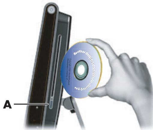
To eject a disc, make sure the power is turned on and then press the eject button (**A**) on the side of the disc drive. You can also tap the **Windows Vista start button**, tap **Computer**, press and hold (or with the mouse, right-click) the CD drive, and then tap **Eject**.
