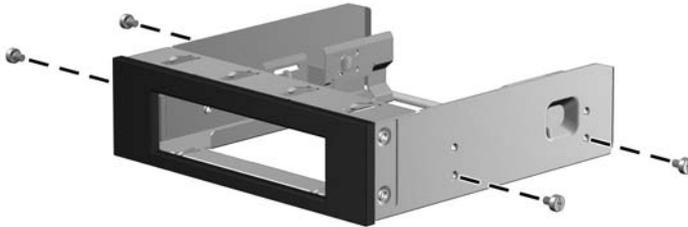
2. To install the media reader in the 5.25-inch optical bay adapter:
