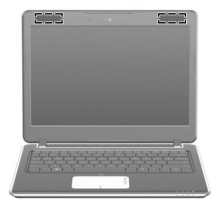
NOTE: For optimal transmission, keep the areas immediately around the antennae free from obstructions.
