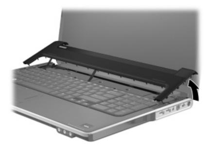
5. Lift the switch cover (1) to access the keyboard screws.
