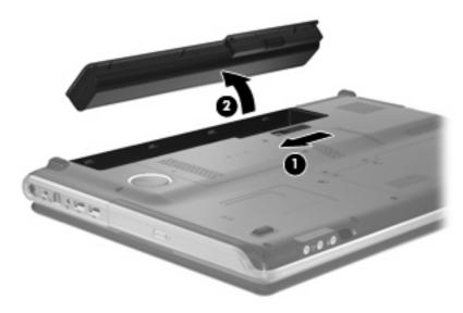
To insert the battery, insert the rear edge of the battery into the battery bay and pivot the front edge of the battery downward until it is seated. The battery release latch automatically locks the battery into place.
