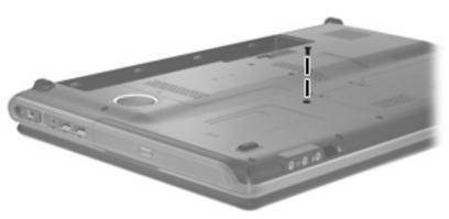
Where used: One screw that secures the optical drive to the computer
