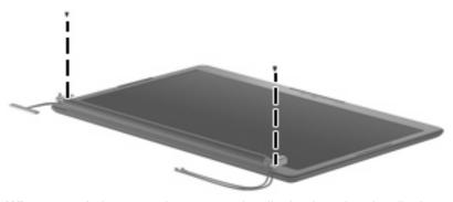
Where used: 2 screws that secure the display bezel to the display enclosure on computer models equipped with BrightView display assemblies
