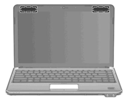
NOTE: For optimal transmission, keep the areas immediately around the antennae free from obstructions.
