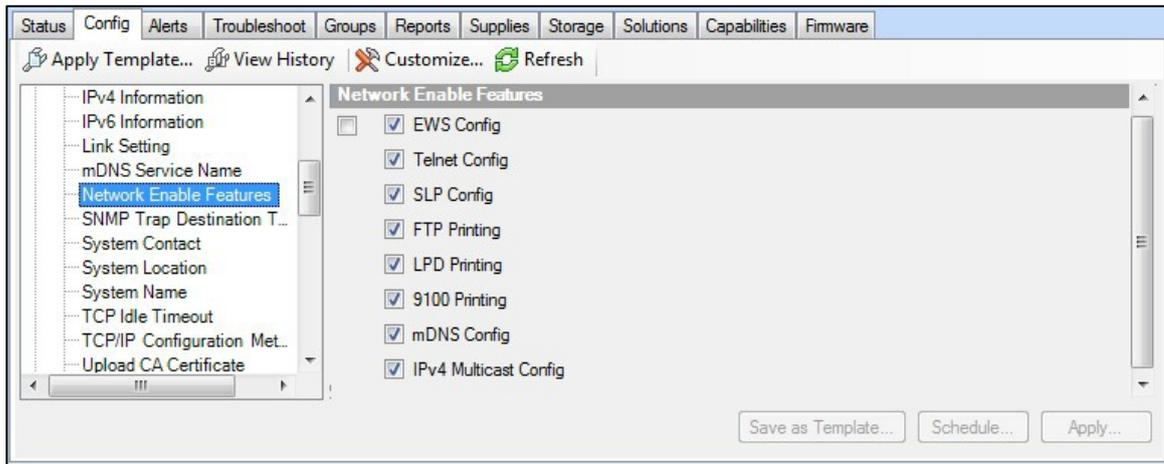
In the HP DesignJet T830 MFP/T730 printer and HP DesignJet T200/600/Studio Printer, the network Management Protocols can be configured from the **Network > Advanced Settings** menu.
