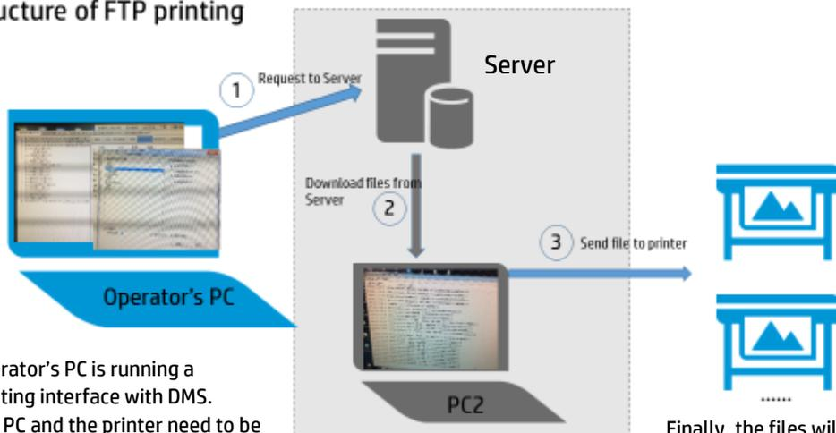
Operator's PC is running a printing interface with DMS. The PC and the printer need to be in the same intranet. List all the jobs from DMS that need to be printed. When the operator clicks print, and selects the printer, a request
