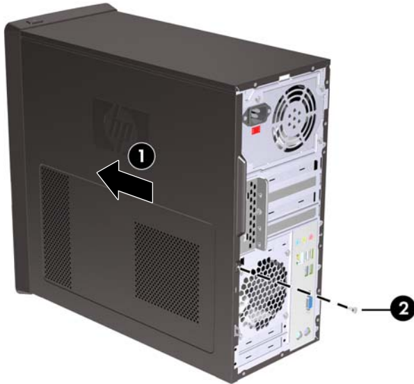
Figure 2-2 Replacing the Computer Access Panel
