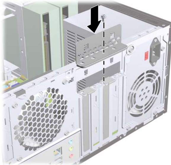
Figure 2-14 Securing the Expansion Cards and Slot Covers
