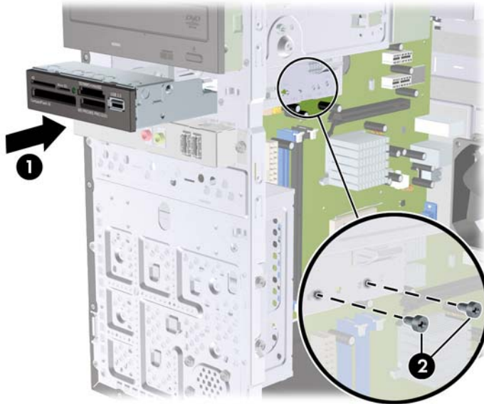
Figure 2-25 Installing a 3.5-inch Device (Media Card Reader Shown)
