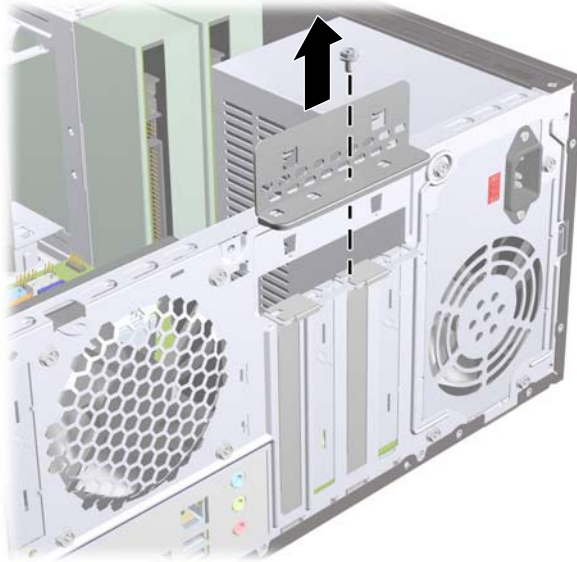
Figure 2-9 Opening the Slot Cover Lock
