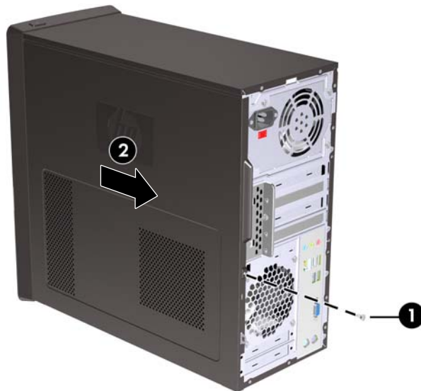
Figure 2-1 Removing the Computer Access Panel
