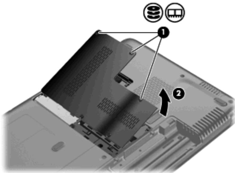
9. Loosen the 2 captive screws that secure the hard drive to the computer **(1)**.
