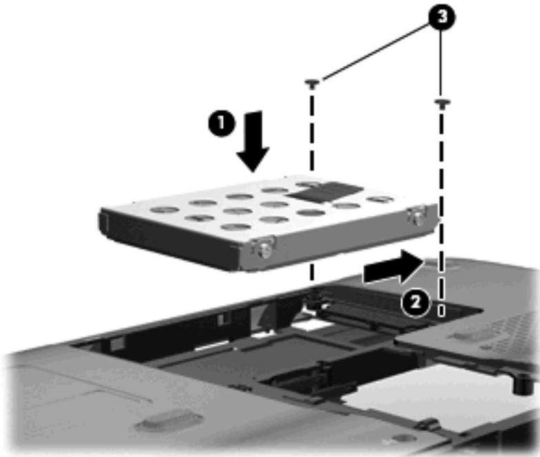
4. Align the tabs on the hard drive cover with the notches on the computer (1).
