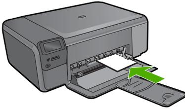
3. Slide the paper-width guide inward until it stops at the edge of the paper. Do not overload the paper tray; make sure the stack of paper fits within the paper tray and is no higher than the top of the paper-width guide.
