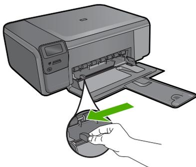
2. Insert the stack of photo paper into the far-right side of the paper tray with the short edge forward and the print side down. Slide the stack of photo paper forward until it stops.
