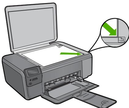
The product aligns the print cartridges. Recycle or discard the print cartridge alignment sheet.
