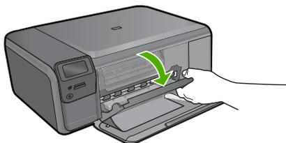
3. Wait until the print carriage is idle and silent, and then lightly press down on a print cartridge to release it.
