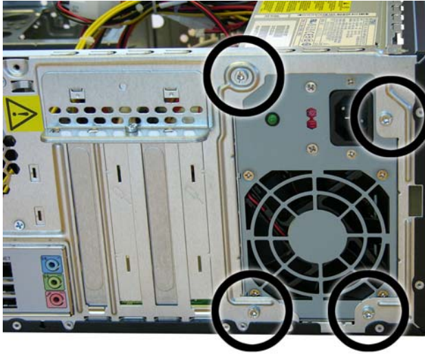
Figure 6-41 Removing the power supply screws
