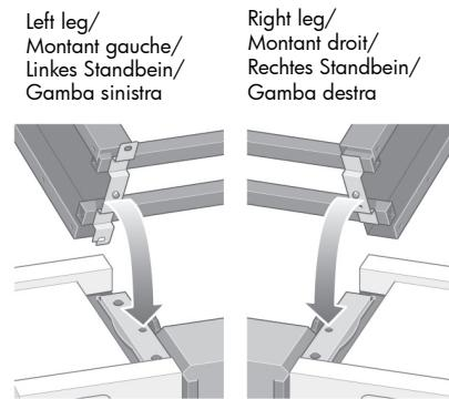
Advance warning: in the next step, make sure you position the stand pins in the holes in the center of the printer body brackets.
