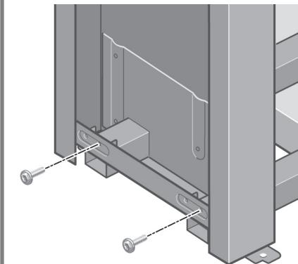
Fix the left leg to the cross-brace using two screws on the outer side of the leg.
