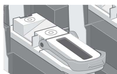
Before removing the setup printheads, look at the window on top of each one and check that the printhead contains ink.
