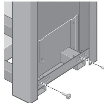
Fix the right leg to the cross-brace using two screws on the outer side of the leg.
