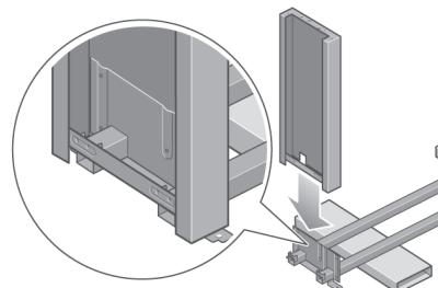
Lower the left leg onto the left side of the cross-brace. The left leg will fit only on the left side of the cross-brace.
