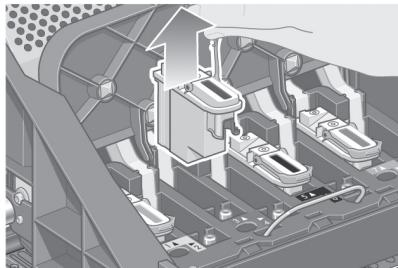
Lift the setup printhead until it is released from the carriage assembly. Then remove the other setup printheads.
