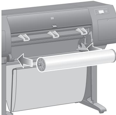
With the blue stop on the left, slide the spindle into the printer. The blue spindle lever will drop down automatically as you insert the spindle.
