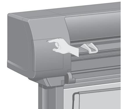
Find the ink cartridge door, which is on the left side of the printer.
