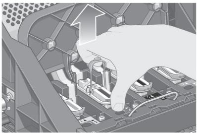
Using the blue handle, gently disengage the setup printhead from the carriage.
