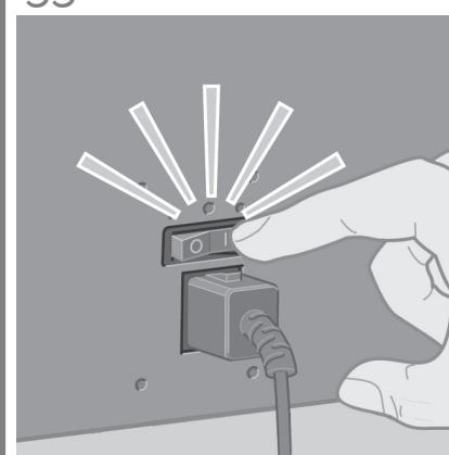
Turn the power switch at the rear of the printer to the on position.
