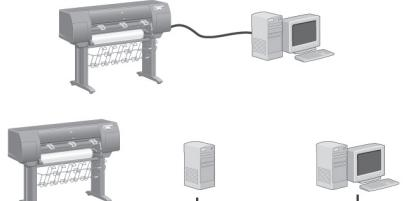
Your printer can be connected to a computer directly or to one or more computers via a network.
