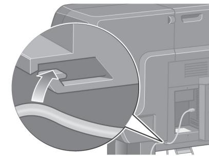
Pass the LAN cable through the hook at the rear of the printer.
