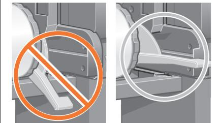
The spindle lever will be in the horizontal position when the spindle has been correctly inserted.
