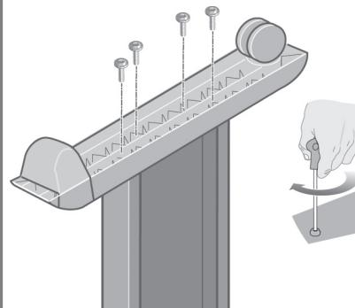
Fix the right foot using four screws.
