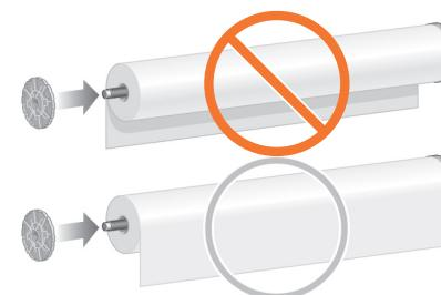
Slide a roll of paper onto the spindle. Make sure the paper is oriented exactly as shown.
