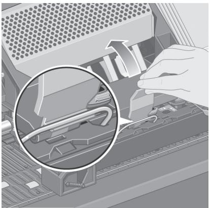
Make sure the latch engages correctly
