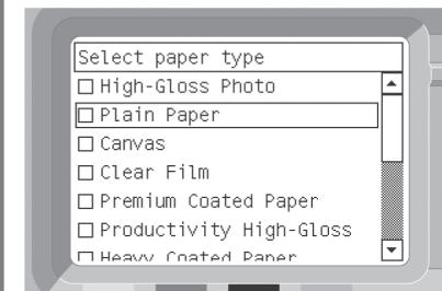
The front panel displays the above. Highlight the paper type you have loaded and press the Select (✓) key.
