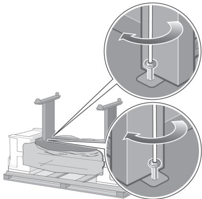
Fix the left side of the stand to the printer using two screws. Make sure that the screws are fully tightened.
