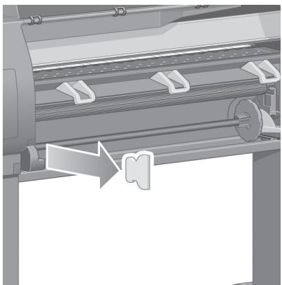
Remove the spindle lock foam piece.
