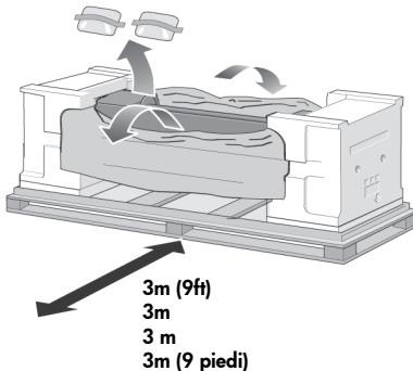
Pull open the protective plastic from the base of the printer. Please ensure that there is a three-meter space clear of obstructions to the rear of the printer. Remove the two desiccant bags from the printer.
