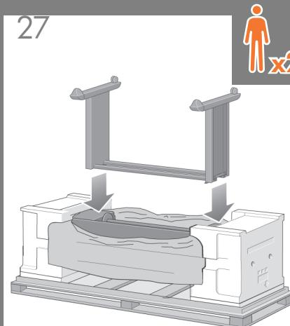
Lift the stand assembly onto the printer body. The anti-slip material should face to the rear of the printer.
