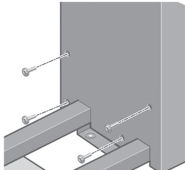
Fix the right leg to the cross-brace using four screws on the inner side of the leg.
