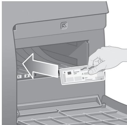
Insert the printhead cleaner into the slot of the correct color.
