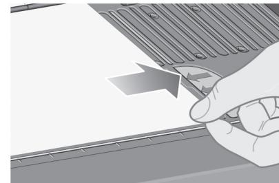
Make sure the paper is aligned with the blue line and half circle on the platen.
