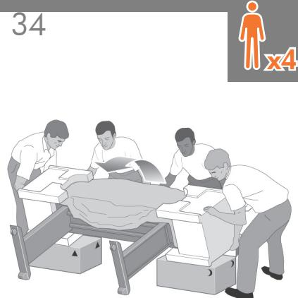
Using four people and the hand holds on the rear of the printer body, carefully lift the printer into an upright position.
