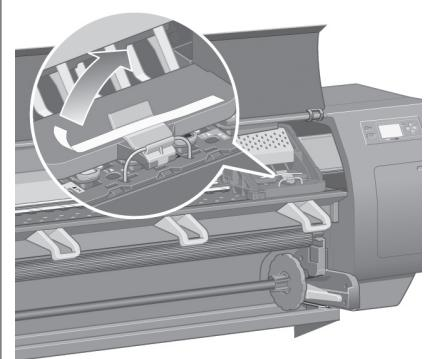
Remove the packing tape that is holding down the printhead carriage latch.
