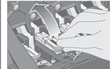
To remove a setup printhead, lift up the blue handle.
