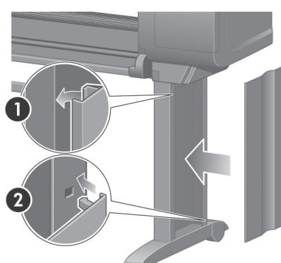
Position the right leg cover on the front of the right leg (1), then clip the rear edge (2) into place.
