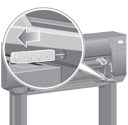
Remove the spindle lock.
