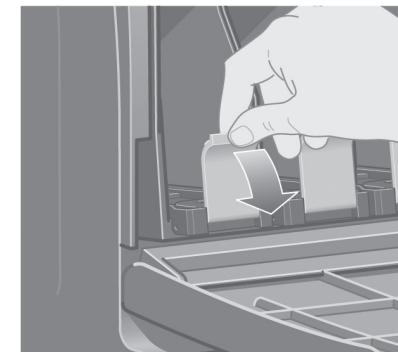
To release the ink cartridge drawer, pull the blue handle down.
