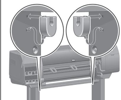
Attach the two plastic brackets to the top part of the printer legs. Insert the tab at the bottom of the bracket into the leg, and then 'click' the top of the bracket into place.
