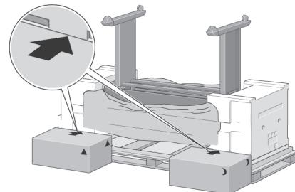
Place the spare and consumables boxes against the rear of the printer box. The arrows on the boxes must point towards the printer box. Check that the anti-slip material is still fixed to the two rear wheels.
