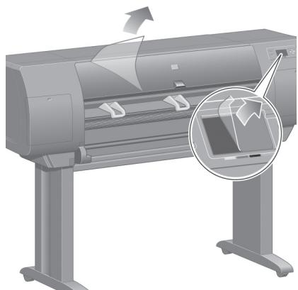
Remove the protective covering from the printer window and the front panel screen.
