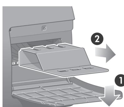
Open the printhead cleaner door and remove the carriage packing material. Then close the cleaner door.
