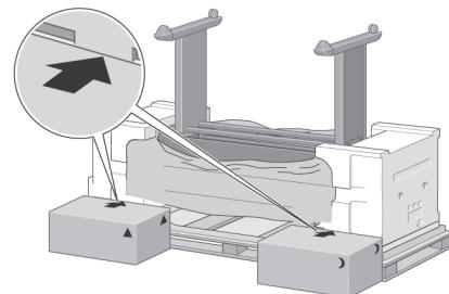
Place the spare and consumables boxes against the rear of the printer box. The arrows on the boxes must point towards the printer box. Check that the anti-slip material is still fixed to the two rear wheels.
