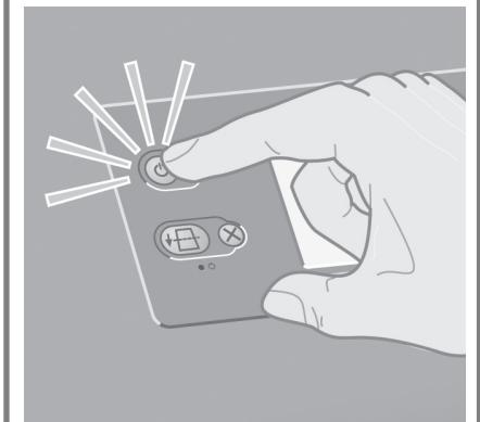
If the power light on the front panel remains off, press the Power key to switch on the printer.
