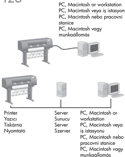
Your printer can be connected to a computer directly or to one or more computers via a network.
