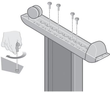
Fix the left foot using four screws.
