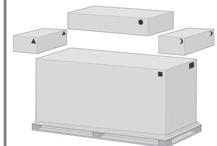
Remove the boxes from the top of the main printer box.
