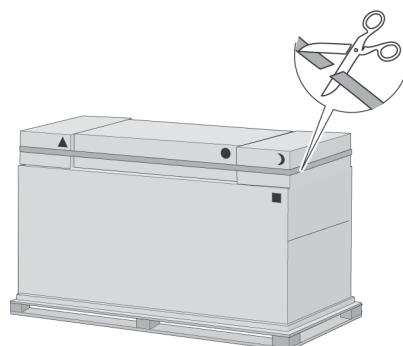
Cut the strap around the boxes carefully, as the boxes may fall as soon as the strap is cut.
