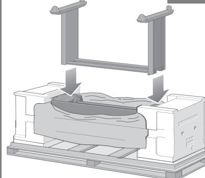
Lift the stand assembly onto the printer body. The anti-slip material should face to the rear of the printer.
