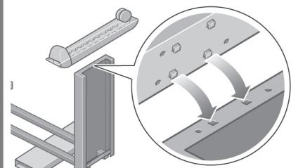
Position a foot on the right leg. There are pins to help you to position the foot correctly. Do not remove the anti-slip material from the wheel.
