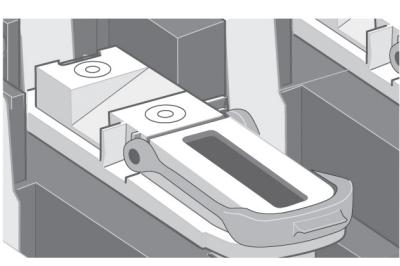
Before removing the setup printheads, look at the window on top of each one and check that the printhead contains ink.
