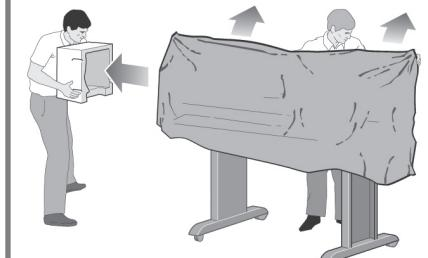
Remove the two foam end packs and the plastic covering the printer.
