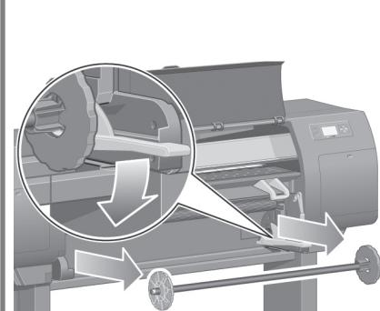
Press the spindle lever down, which will unseat the right-hand end of the spindle. Remove that end of the spindle first, and then the left.
