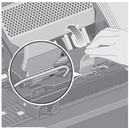
Make sure the latch engages correctly.
