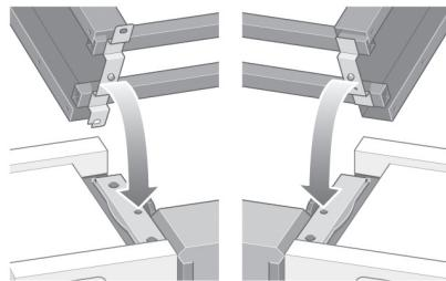
Advance warning: in the next step, make sure you position the stand pins in the holes in the center of the printer body brackets.
