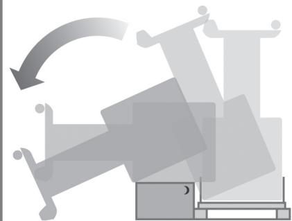
Rotate the printer until its rear rests on the spare and consumables boxes and the wheels with the anti-slip material touch the floor.
