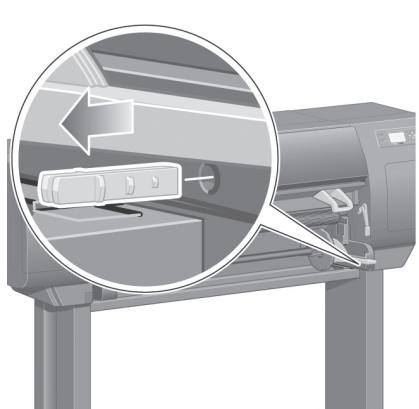
Remove the spindle lock.
