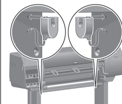
Attač the two plastic brackets to the top part of the printer legs. Insert the tab at the bottom of the bracket into the leg, and then 'click' the top of the bracket into place.
