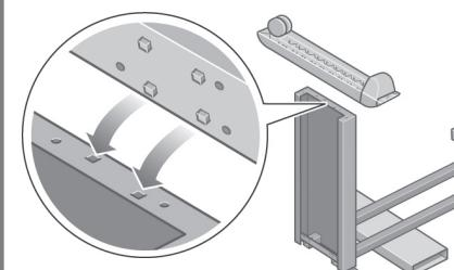
Position a foot on the left leg. There are pins to help you to position the foot correctly. Do not remove the anti-slip material from the wheel.
