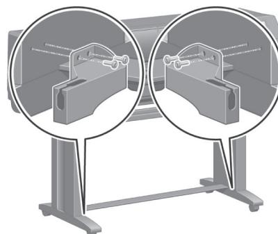
Use four screws to attach the brackets to the lower part of the printer legs. (Each bracket requires two screws.)
