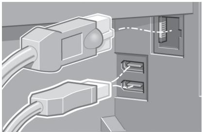
A Gigabit Ethernet socket is provided for connection to a network. Two FireWire sockets are provided for direct connection to computers.
