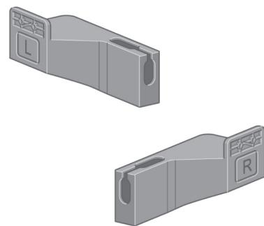
Remove the two brackets from the box that contains the stand and the bin. Note: The brackets are marked L and R.
