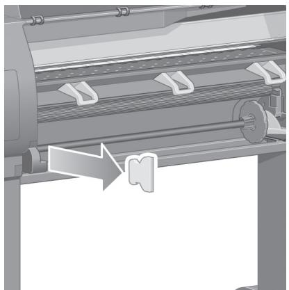
Remove the spindle lock foam piece.
