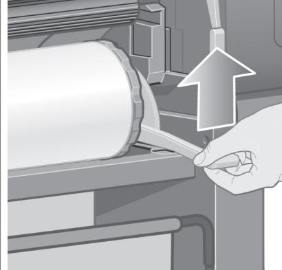
Once you meet resistance, lift the blue lever to seat the spindle properly.
