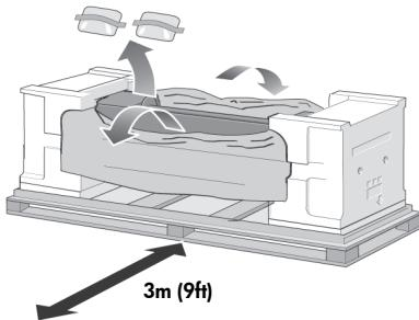
Pull open the protective plastic from the base of the printer. Please ensure that there is a three-meter space clear of obstructions to the rear of the printer. Remove the two desiccant bags from the printer.
