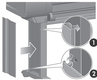
Position the left leg cover on the front of the left leg (1), then clip the rear edge (2) into place.
