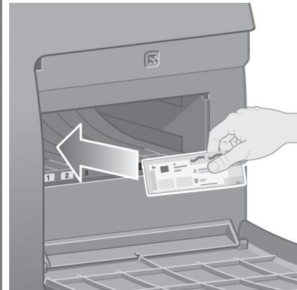
Insert the printhead cleaner into the slot of the correct color.
