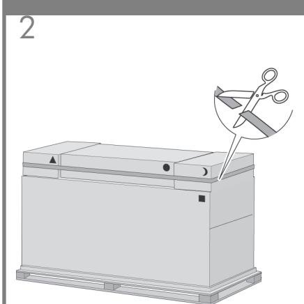
Cut the strap around the boxes carefully, as the boxes may fall as soon as the strap is cut.
