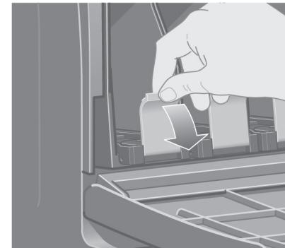
To release the ink cartridge drawer, pull the blue handle down.
