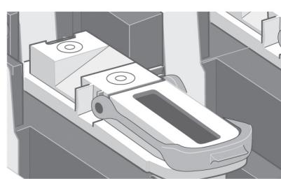
Before removing the setup prinheads, look at the window on top of each one and check that the printhead contains ink.
