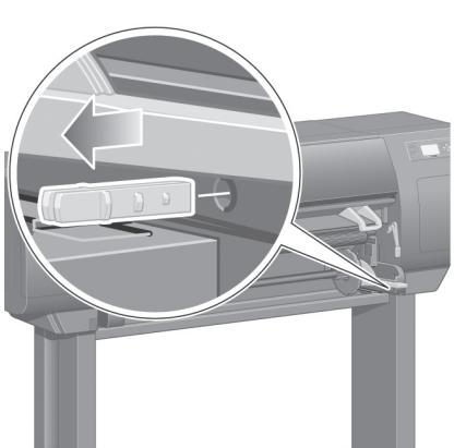
Remove the spindle lock.
