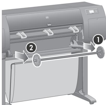
Remove the right-hand end of the spindle (1) from the printer, then move it to the right in order to extract the other end (2).
