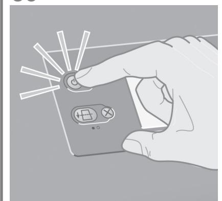
If the power light on the front panel remains off, press the Power key to switch on the printer.
