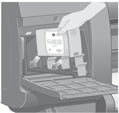
Place the ink cartridge onto the ink cartridge drawer. Note that there are marks on the drawer showing the correct location.
