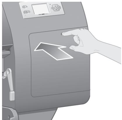
Press the printhead cleaner door, which is on the right side of the printer.
