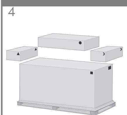
Remove the boxes from the top of the main printer box.
