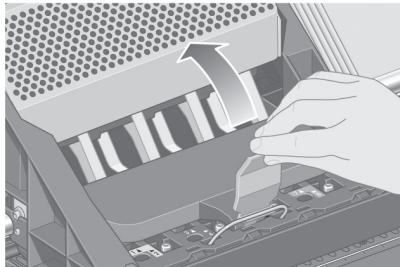
Lift up the cover. This will give you access to the setup printheads.
