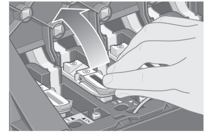
To remove a setup printhead, lift up the blue handle.
