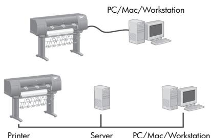
Your printer can be connected to a computer directly or to one or more computers via a network.
