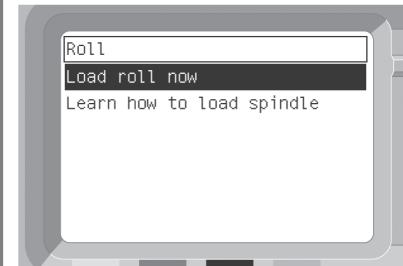
The front panel displays the above. Highlight 'Load roll now' and press the Select (✓) key.
