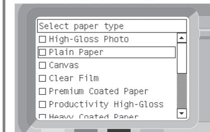
The front panel displays the above. Highlight the paper type you have loaded and press the Select (✓) key.
