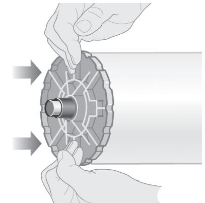
Put the blue-colored stop onto the spindle and push it on as far as it will go without using excessive force.
