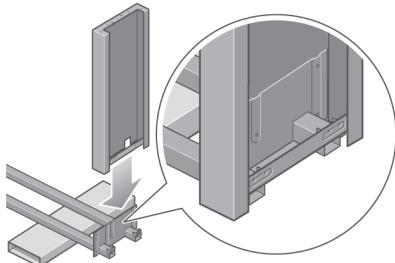
Lower the right leg onto the right side of the cross-brace. The right leg will fit only on the right side of the cross-brace.
