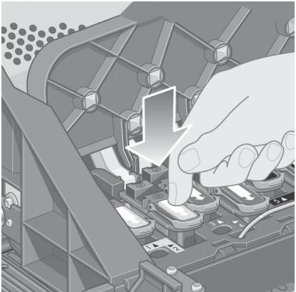
Make sure the printheads are correctly seated. When all the printheads are installed, the front panel prompts, "Close printhead cover and window".
