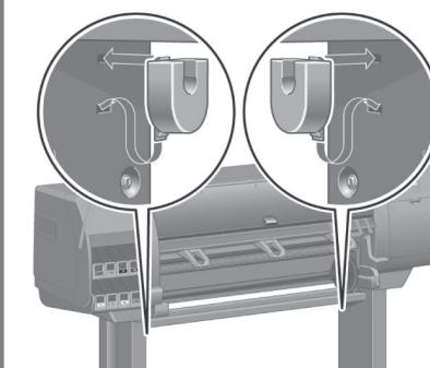
Attach the two plastic brackets to the top part of
