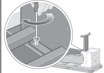
Fix the right side of the stand to the printer using one screw. Make sure that the screw is fully tightened.
