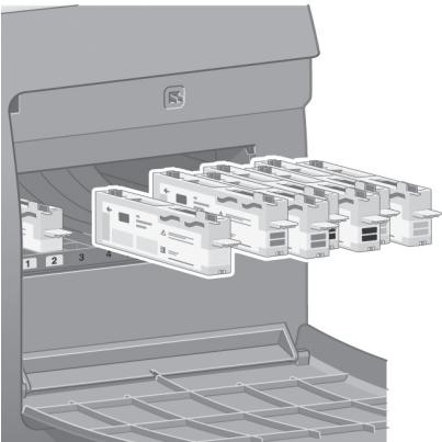
Insert the other seven printhead cleaners into the correct slots.
