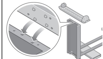
Position a foot on the left leg. There are pins to help you to position the foot correctly. Do not remove the anti-slip material from the wheel.
