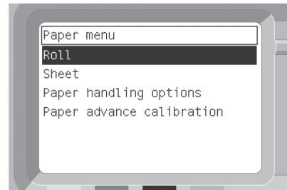
From the front panel, highlight 'Roll' and press the Select (✓) key.
