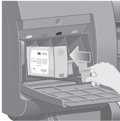
Push the ink cartridge drawer back into the printer until it locks into position.
