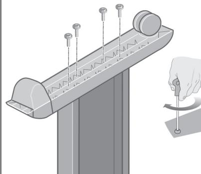
Fix the right foot using four screws.
