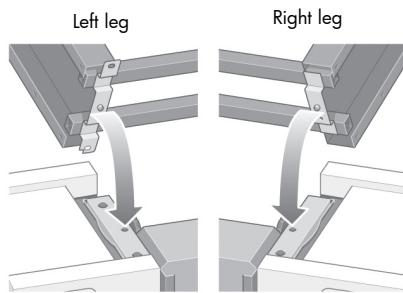
Advance warning: in the next step, make sure you position the stand pins in the holes in the center of the printer body brackets.
