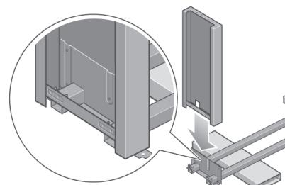
Lower the left leg onto the left side of the cross-brace. The left leg will fit only on the left side of the cross-brace.
