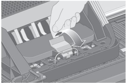
Pull up and release the latch on top of the carriage assembly.
