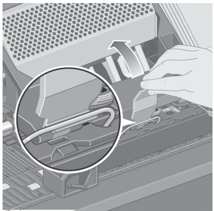
Make sure the latch engages correctly.
