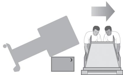
Remove the pallet before trying to lift the printer into an upright position.
