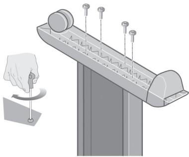
Fix the left foot using four screws.
