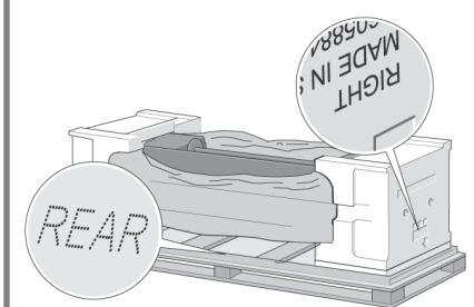
You now need to identify the left and right of the printer. This information is shown on the foam end packs. Also identify the rear of the printer.
