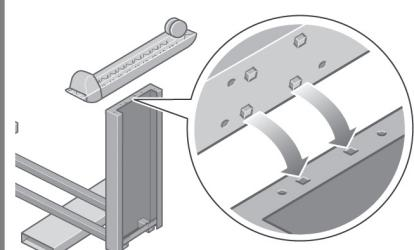
Position a foot on the right leg. There are pins to help you to position the foot correctly. Do not remove the anti-slip material from the wheel.
