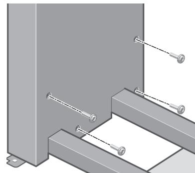
Fix the left leg to the cross-brace using four screws on the inner side of the leg.
