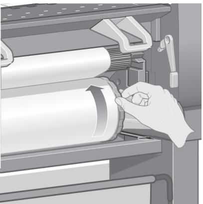
Using the stops, carefully wind the excess paper back on to the spindle.
