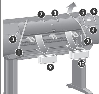
Remove the packing tapes 1 to 8. Open the printer window and remove the two window inserts 9 and 10.
