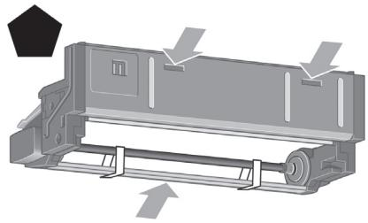
Before unpacking the roll module, note that you should only handle this piece of equipment using the points indicated by the green arrows shown above.
