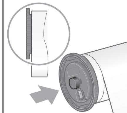
Push the blue left-hand stop onto the roll. Make sure it is correctly seated.
