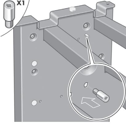
Locate the pin into the left leg.
