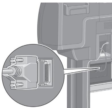
The roll module provides an extra socket to connect an optional accessory.
