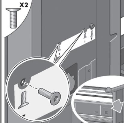
Fix the roll module to the right leg of the stand using two additional screws.
