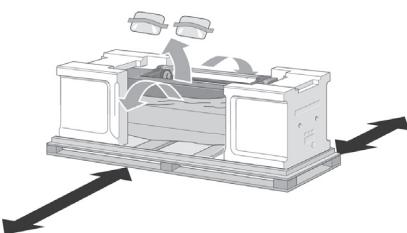
Pull open the protective plastic from the base of the printer. Please ensure that there is a three-meter space clear of obstructions to the rear of the printer and one meter at the front of the printer.
