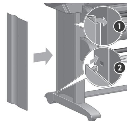
Position the left leg cover on the front of the left leg (1), then clip the rear edge (2) into place.
