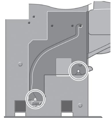
Before the roll module is moved into its final position, please note that the roll module should sit on the pins that were located on the stand legs earlier.
