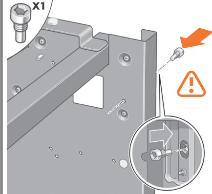
Locate the pin into the interior of the right leg.
