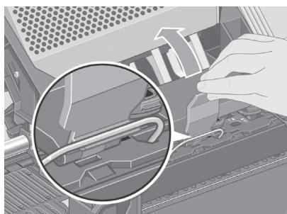
Make sure the latch engages correctly.
