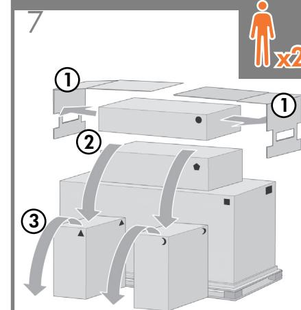
Remove the 2 lids. Place the consumables and spare boxes in front of the printer body. Then lower the stand and bin box onto the consumables and spare boxes.
