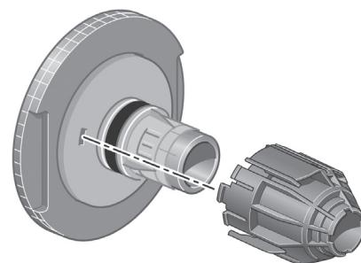
Shown above is one of the core adaptors supplied. Use these when the roll core is of a larger diameter.
