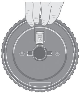
As shown above, hold the spindle assembly using the blue and black stops.
