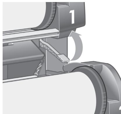
Lift the blue lever on Drawer 2. This is located on the right-hand side of the printer and under Drawer 1.
