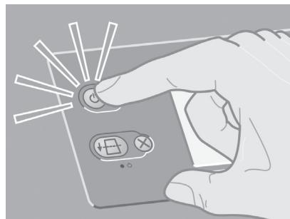
If the power light on the front panel remains off, press the Power key to switch on the printer.
