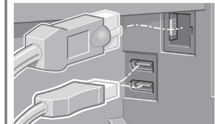
A Gigabit Ethernet socket is provided for connection to a network.
