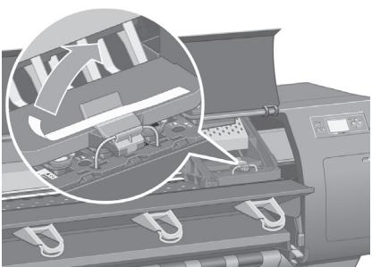
Remove the packing tape that is holding down the printhead carriage latch.
