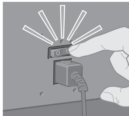
Turn the power switch at the rear of the printer to the on position.
