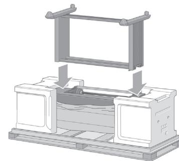
Lift the stand assembly onto the printer body. The anti-slip material should face to the rear of the printer.
