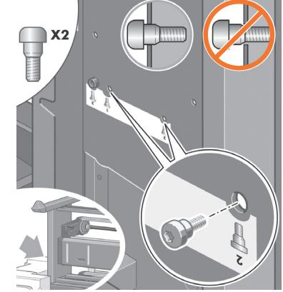
Fix the roll module to the left leg of the stand using two collar-headed screws.
