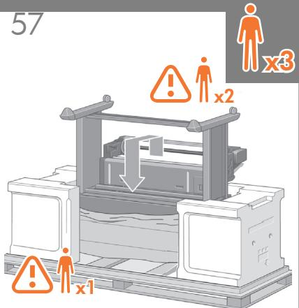
Three people are needed, two at the front and one at the rear of the printer. The two at the front should lift the roll module and then, with the help of the third person at the rear, lower it vertically onto the pins located earlier on the stand.
