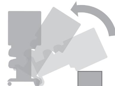
Rotate the printer into an upright position. The anti-slip material should stop the printer from sliding forwards.
