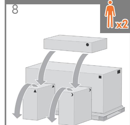
Lower the roll module box onto the consumables and spare boxes. Then lower the roll module box onto the floor. Then remove the consumables and spare boxes.
