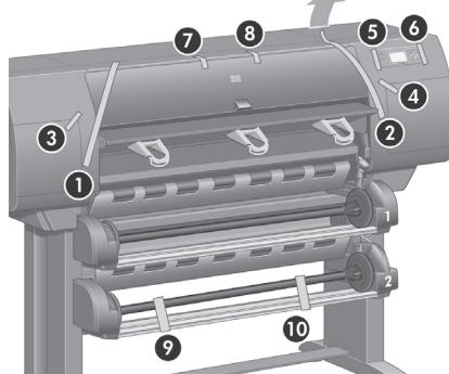
Remove the packing tapes 1 to 10.
