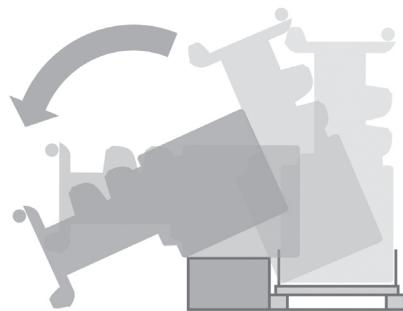
Rotate the printer until its rear rests on the spare and consumables boxes and the wheels with the anti-slip material touch the floor.
