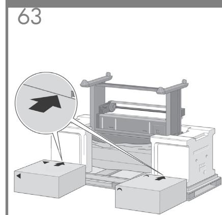
Place the spare and consumables boxes against the rear of the printer box. The arrows on the boxes must point towards the printer box. Check that the anti-slip material is still fixed to the two rear wheels.
