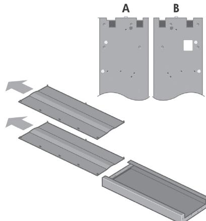
Identify the left leg (A) and the right leg (B) as shown above. Remove the two leg covers from the left leg.
