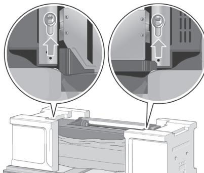
Using the screwdriver supplied, remove the two screws that hold Drawer 1 in place. Note: the screws are only for transit, they are not to be replaced.
