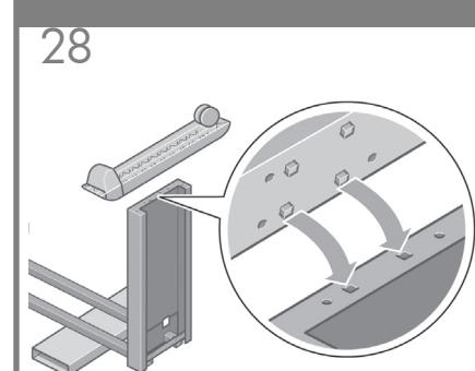
Position a foot on the right leg. There are pins to help you to position the foot correctly. Do not remove the anti-slip material from the wheel.
