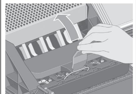
Lift up the cover. This will give you access to the setup printheads.
