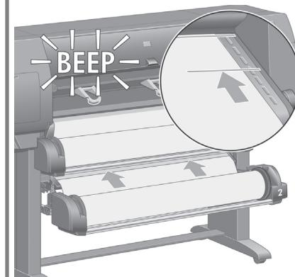
Feed the paper for a few centimeters more after the printer beeps, then turn the roller backwards to tension the paper correctly.
