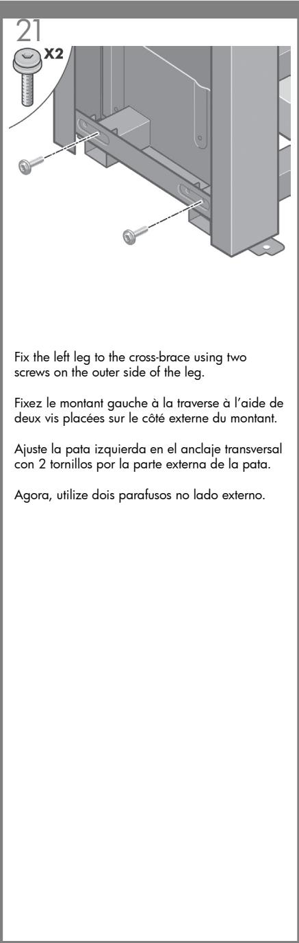
Fix the left leg to the cross-brace using two screws on the outer side of the leg.
