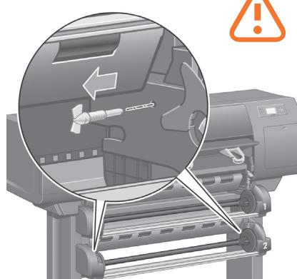
Remove the two yellow plastic screws from the left and right side of Drawer 2. Caution: Be very careful when removing.
