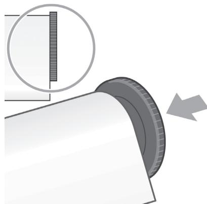
Push the black right-hand stop onto the roll. Make sure it is correctly seated.
