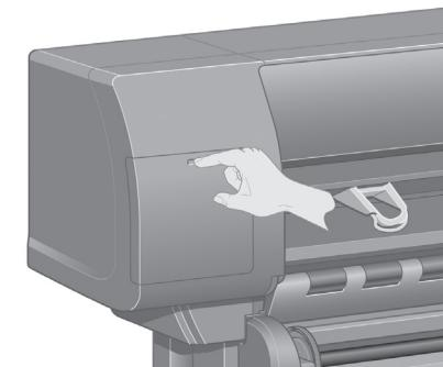
Find the ink cartridge door, which is on the left side of the printer.
