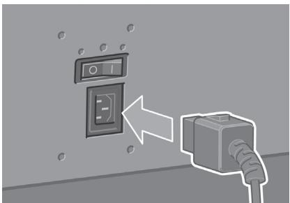
Plug the power cable into the rear of the printer, then plug the other end into the AC power outlet.
