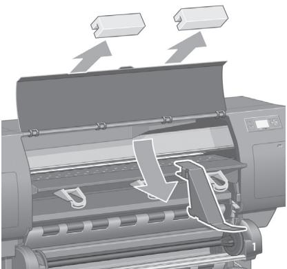
Open the printer window. Then remove the two window inserts and the ink tube packing material.
