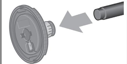
Remove the blue-colored stop from the left end of the spindle. Keep the spindle horizontal.
