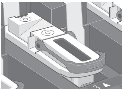
Before removing the setup printheads, look at the window on top of each one and check that the printhead contains ink.
