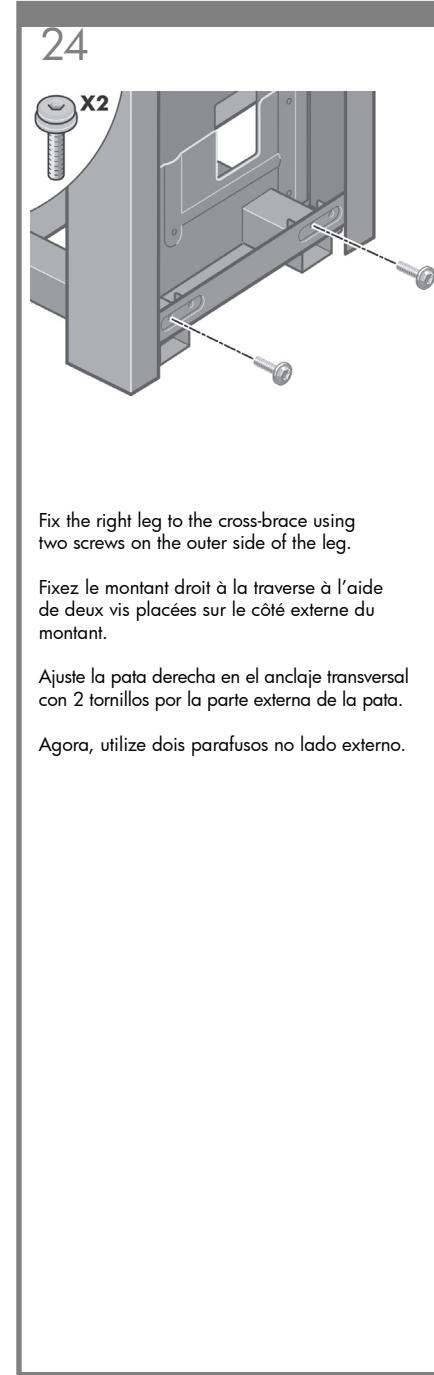
Fix the right leg to the cross-brace using two screws on the outer side of the leg.
