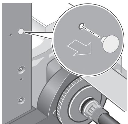
Remove the remaining two yellow plugs from the left and right legs. It is important to remember the positions of these holes.
