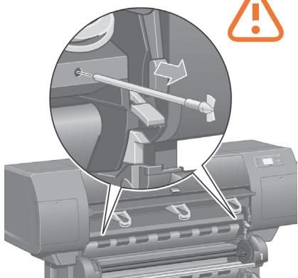
Remove the two yellow plastic screws from the right and left side of the paper feed.
