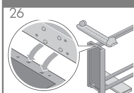
Position a foot on the left leg. There are pins to help you to position the foot correctly. Do not remove the anti-slip material from the wheel.
