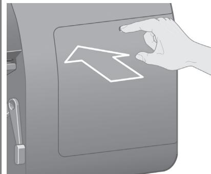
Press the printhead cleaner door, which is on the right side of the printer.
