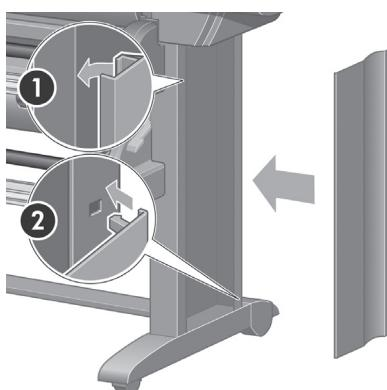
Position the right leg cover on the front of the right leg (1), then clip the rear edge (2) into place.
