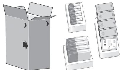
Remove the printheads, printhead cleaners, and ink cartridges from the consumables box.
