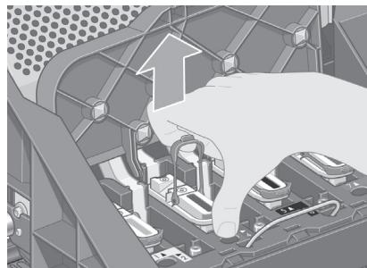
Using the blue handle, gently disengage the setup printhead from the carriage.
