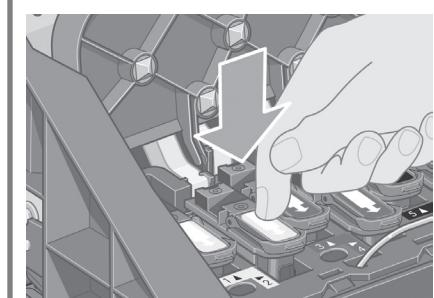
Make sure the printheads are correctly seated. When all the printheads are installed, the front panel prompts, "Close printhead cover and window".
