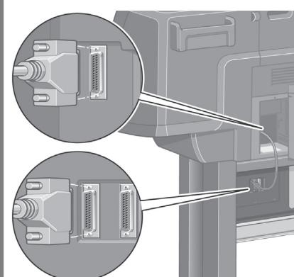
Using the cable supplied, connect the roll module to the printer.
