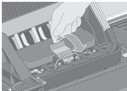
Pull up and release the latch on top of the carriage assembly.
