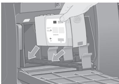
Place the ink cartridge onto the ink cartridge drawer. Note that there are marks on the drawer showing the correct location.
