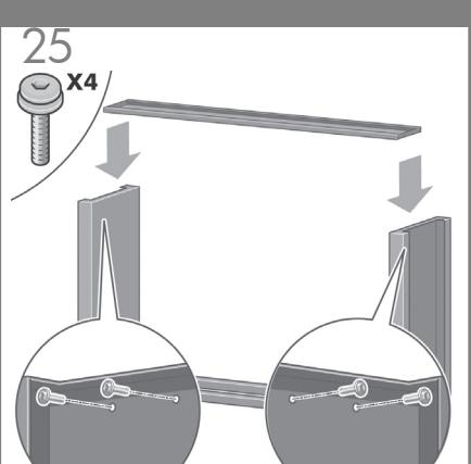
Fix the stand cross-bar using four screws.
