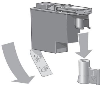
Remove the blue protective cap and the clear protective tape from the printhead.
