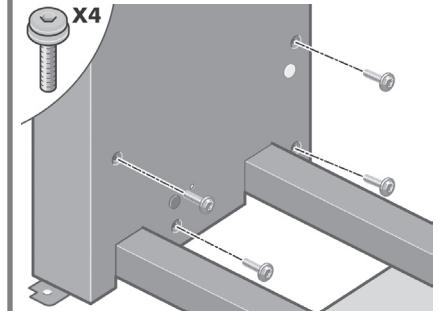
Fix the left leg to the cross-brace using four screws on the inner side of the leg.
