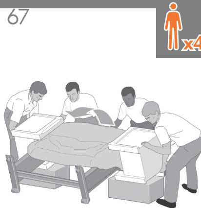
Using four people and the hand holds on the rear of the printer body, carefully lift the printer into an upright position.
