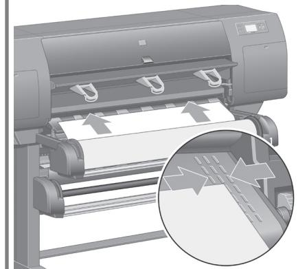
Feed the paper from roll 1 onto the drawer 1 platen. Align the paper parallel with the blue lines on the right side of the platen.
