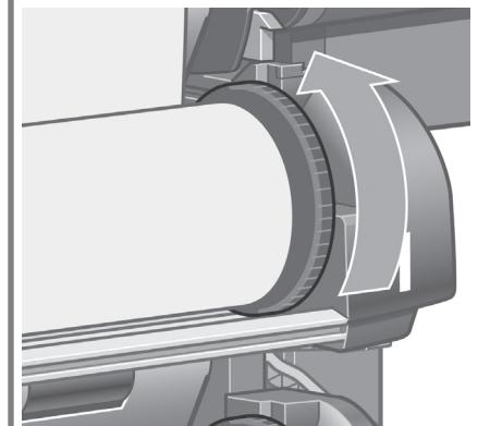
Using the stops, carefully wind the excess paper back on to the spindle.
