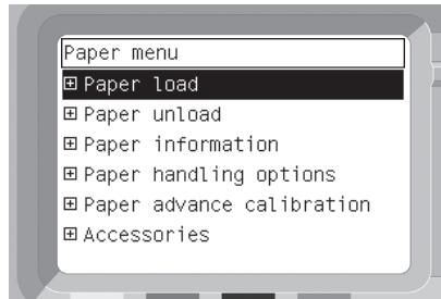
From the front panel, highlight 'Paper load' and press the Select key.
