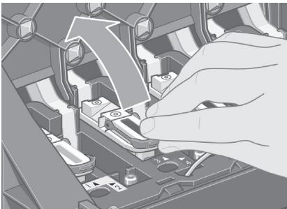
To remove a setup printhead, lift up the blue handle.
