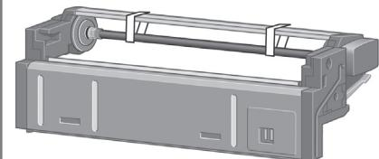
Turn the roll module over into an inverted position as shown above. Then carry it to the front of the inverted printer.
