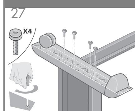
Fix the left foot using four screws.
