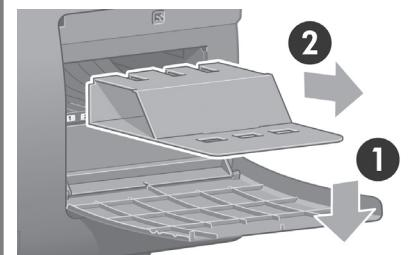
Open the printhead cleaner door and remove the carriage packing material. Then close the cleaner door.
