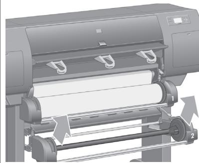
Remove the spindle from Drawer 2.
