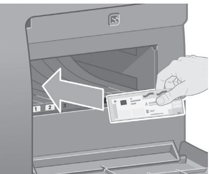
Insert the printhead cleaner into the slot of the correct color.
