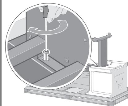
Fix the right side of the stand to the printer using one screw. Make sure that the screw is fully tightened.
