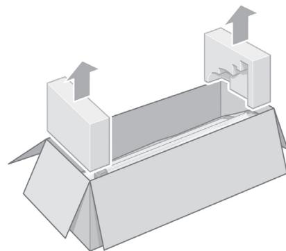
Open the box containing the roll module, then remove the two foam supports.
