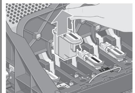
Lift the setup printhead until it is released from the carriage assembly. Then remove the other setup printheads.
