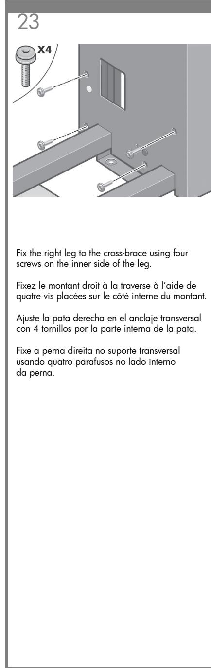
Fix the right leg to the cross-brace using four screws on the inner side of the leg.
