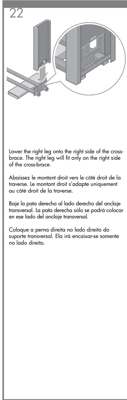
Lower the right leg onto the right side of the cross-brace. The right leg will fit only on the right side of the cross-brace.
