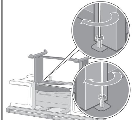
Slide Drawer 1 forwards to gain better access for the front screw. Fix the left side of the stand to the printer using two screws. Make sure that the screws are fully tightened.
