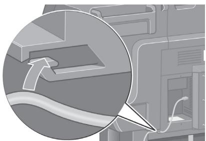
Pass the LAN cable through the hook at the rear of the printer.
