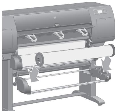
With the blue stop on the left, lower the spindle into Drawer 2.
