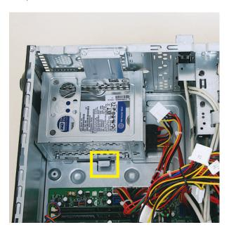
13 Press the cage latch (1), and slide the hard disk drive cage toward the top of the computer (2) to release it.
