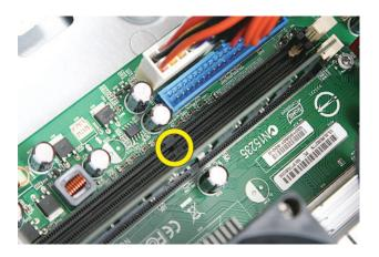
3 Position the memory module over the socket, aligning the notch with the tab in the socket, and then firmly press the module down into the socket...
