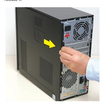
Tilt out the top of the side panel, and then lift the panel from the computer.
