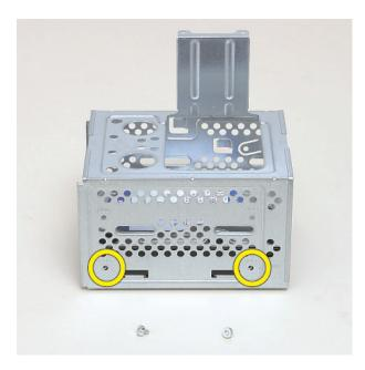
3 Insert and tighten the four screws that secure the drive in the cage.
