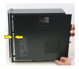
7 Place the bottom of the panel on the computer, inserting the tabs on the inside of the panel into the rail slots on the computer. Swing the top of the panel toward the computer, inserting the top tabs into the rail slots.
