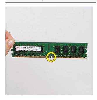
**2** Look at the memory module socket for the tab that matches the notch on the memory module.
