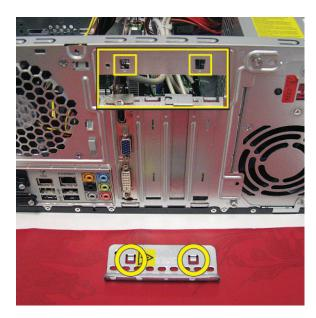
4 Replace the bracket cover onto the back of the computer: Align the bracket cover hooks over the slots on the computer, and then slide the bracket cover into place against the add-in cards.
