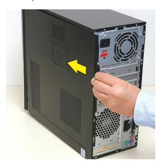
**11** Tighten the side panel thumbscrew on the back of the computer.
