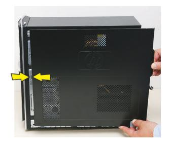
Place the bottom of the panel on the computer, inserting the tabs on the inside of the panel into the rail slots on the computer. Swing the top of the panel toward the computer, inserting the top tabs into the rail slots.
