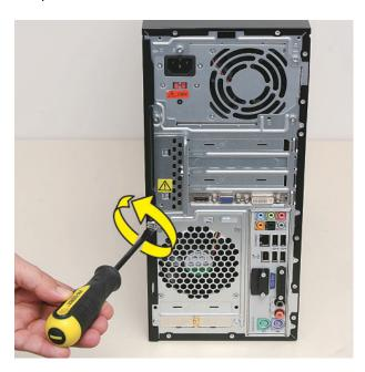
Grasp the handle, and pull the side panel about 2.5 cm (1 inch) toward the back of the computer to release it.
