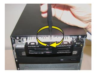
5 Hold the front panel over the front of the computer, and then press the left side of the front panel, inserting the tabs into the computer holes. Swing the right side of the panel toward the computer, inserting the panel tabs, and then press it into the computer.
