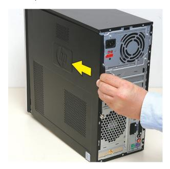
Tighten the side panel thumbscrew on the back of the computer.
