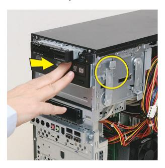
5 Hold the front panel over the front of the computer, and then press the left side of the front panel, inserting the tabs into the computer holes. Swing the right side of the panel toward the computer, inserting the panel tabs, and then press it into the computer.
