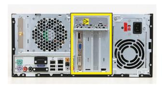
**9** On the back of the computer, remove the screw from the bracket cover for the add-in cards. If it is present, also remove the additional screw that secures a large graphics card.
