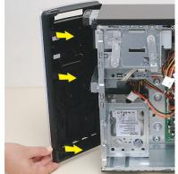
2 Hold the side panel over the side of the computer with the front edge of the panel about 2.5 cm (1 inch) from the front of the computer.
