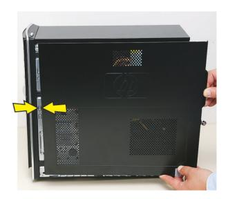
6 Place the bottom of the panel on the computer, inserting the tabs on the inside of the panel into the rail slots on the computer. Swing the top of the panel toward the computer, inserting the top tabs into the rail slots.
