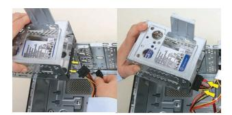
7 Lower the cage into the computer, inserting the four tabs on the bottom of the cage into the computer slots.
