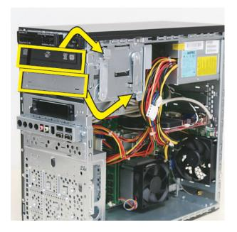
11 Pull out the optical drive latch (1), and then swing it to the left until it is in the center position (2).
