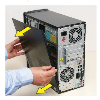
**8** Locate the three tabs that secure the front panel to the computer. Pull each of the tabs out slightly, away from the computer, to release the panel.
