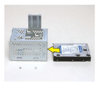
2 Slide the drive into the cage until the four screw holes in the sides of the drive align with the holes in the cage.
