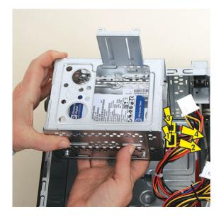
**16** Remove the four screws (two on each side) that secure the drive in the cage.
