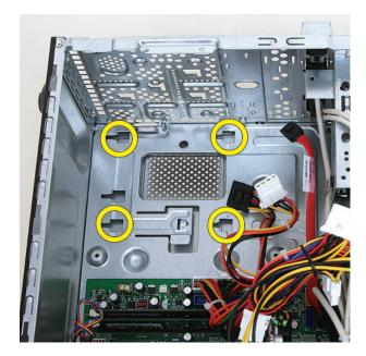
**6** Hold the cage over the computer, and connect the hard disk drive power and data cables.
