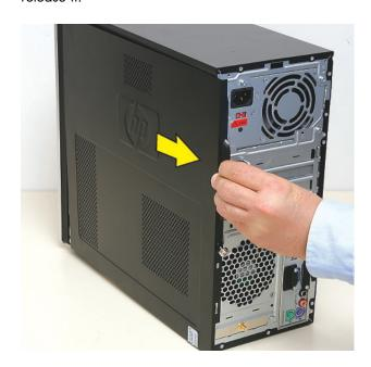
7 Tilt out the top of the side panel, and then lift the panel from the computer.
