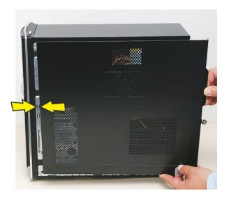
3 Place the bottom of the panel on the computer, inserting the tabs on the inside of the panel into the rail slots on the computer. Swing the top of the panel toward the computer, inserting the top tabs into the rail slots.
