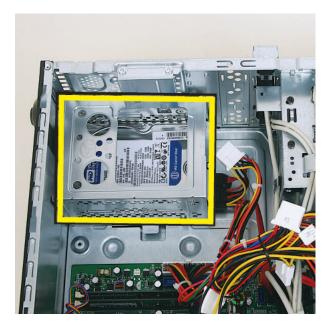
Remove the two screws that secure the hard disk drive cage in the computer.
