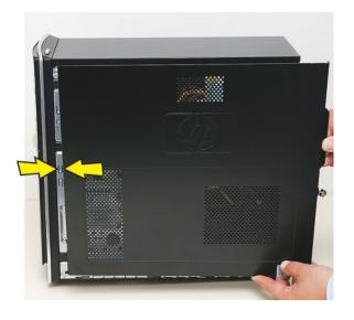
Place the bottom of the panel on the computer, inserting the tabs on the inside of the panel into the rail slots on the computer. Swing the top of the panel toward the computer, inserting the top tabs into the rail slots.
