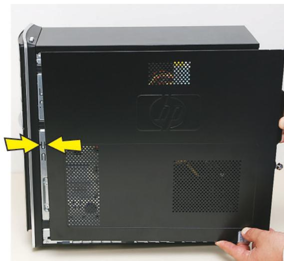
**9** Place the bottom of the panel on the computer, inserting the tabs on the inside of the panel into the rail slots on the computer. Swing the top of the panel toward the computer, inserting the top tabs into the rail slots.
