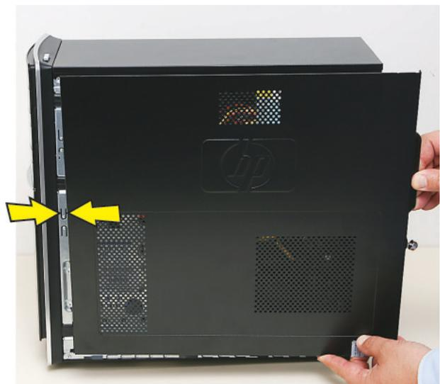
**13** Place the bottom of the panel on the computer, inserting the tabs on the inside of the panel into the rail slots on the computer. Swing the top of the panel toward the computer, inserting the top tabs into the rail slots.
