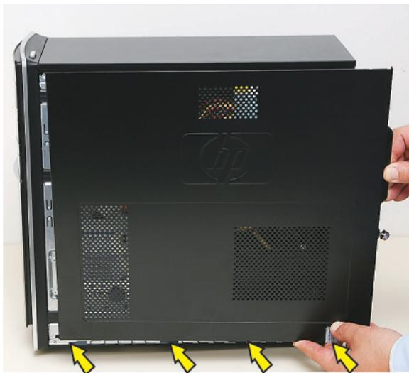
**11** Tighten the side panel thumbscrew on the back of the computer.
