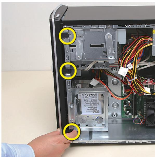
**8** Swing the front panel open toward the left, and then lift it off the computer.
