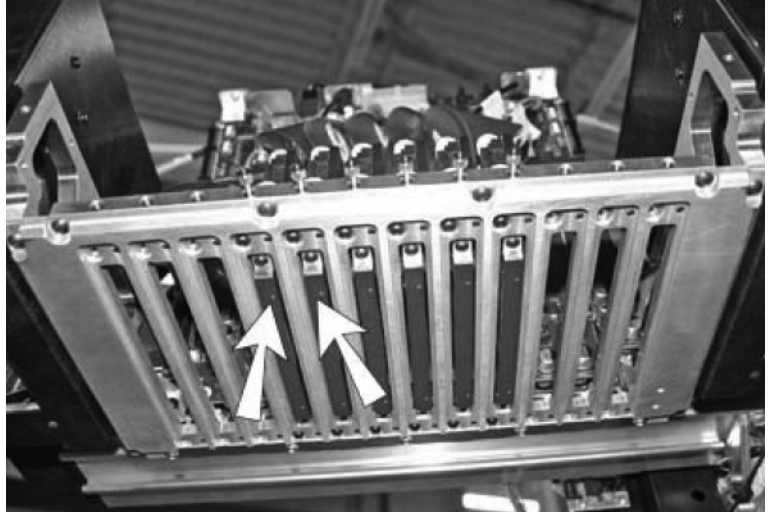
Fig. 4-10. Center the carriage at these two points over the wipers
