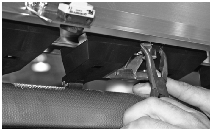
Fig. 4-8. Media thickness sensor (brushes removed for clarity, not necessary to perform procedure)
