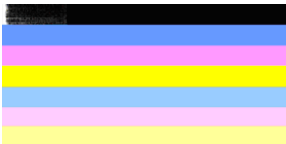
Example of Bad Color Bars The top black bar is ragged on one end.
