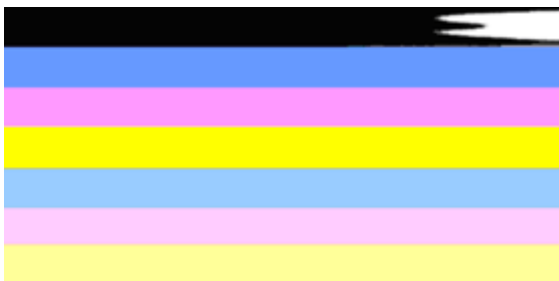
Example of Bad Color Bars The top bar is irregularly streaked or fading.
