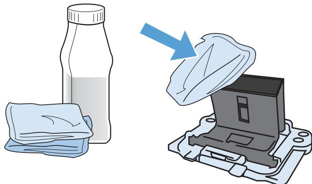
**⚠️ WARNING!** Alcohol is flammable. Keep the alcohol and cloth away from an open flame. Before you close the product and plug in the power cord, allow the alcohol to dry completely.
