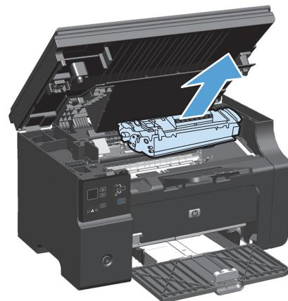
3. Remove the new print cartridge from the packaging. Place the used print cartridge in the bag and box for recycling.
