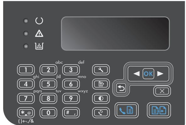
2. Use the arrow buttons to select the **Copy setup** menu, and then press the **OK** button.
