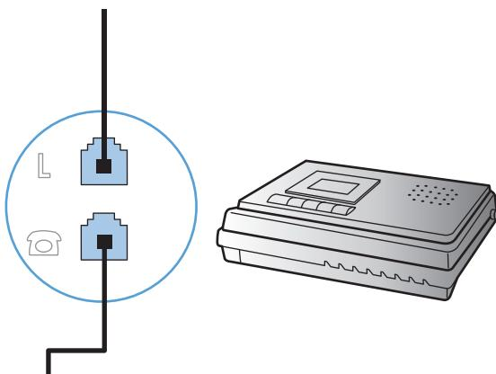
7. To connect a telephone, plug a telephone cord into the previous device's "telephone" port. Plug the other end of the telephone cord into the telephone "line" port.
