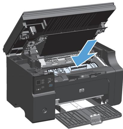
5. Close the print-cartridge door and the scanner assembly.
