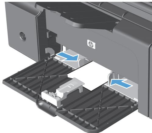
4. Push the paper into the product until it stops, and then slide the front media guide so the tool supports the paper.
