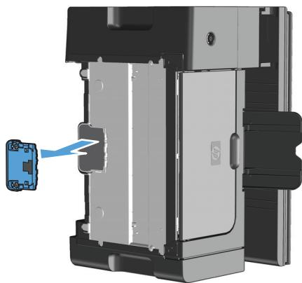
5. Insert the new separation pad, and screw it into place.
