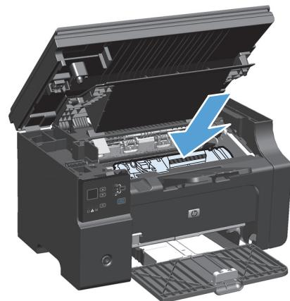
**6.** Close the print-cartridge door and the scanner assembly.
