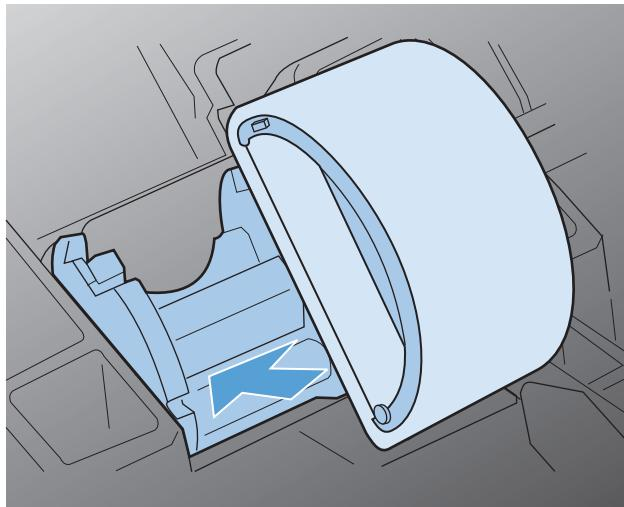
7. Rotate the top of the new pickup roller away from you until both sides snap into place.
