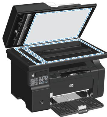
**⚠ CAUTION:** Do not use abrasives, acetone, benzene, ammonia, ethyl alcohol, or carbon tetrachloride on any part of the product; these can damage the product. Do not place liquids directly on the glass or platen. They might seep and damage the product.
