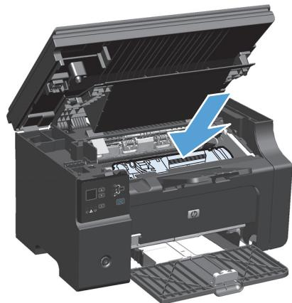
9. Close the print-cartridge door and the scanner assembly.
