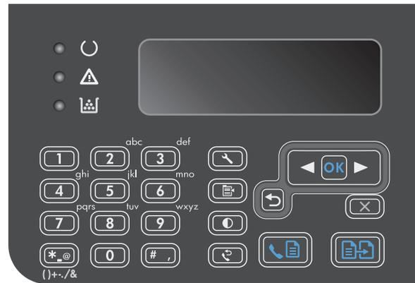
3. Use the arrow buttons to select the correct reduction or enlargement option, and then press the **OK** button.
