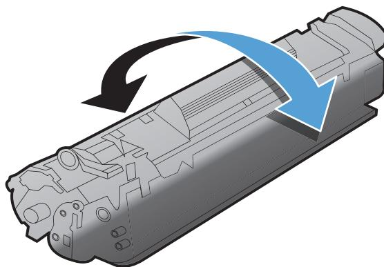
5. Bend the tab on the left side of the cartridge until the tab breaks loose, and then pull the tab until all the tape is removed from the cartridge. Place the tab and tape in the print-cartridge box to return for recycling.
