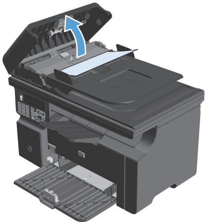
2. Carefully remove jammed paper. Gently try to remove the page without tearing it.
