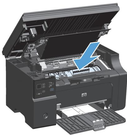
7. Close the print-cartridge door and the scanner assembly.
