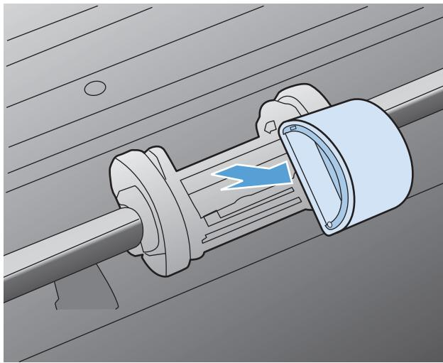
6. Position the new pickup roller in the slot. The circular and rectangular slots on each side prevents you from installing the roller incorrectly.
