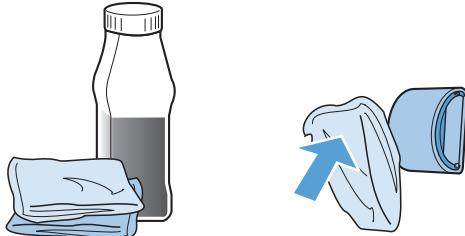
**⚠️ WARNING!** Alcohol is flammable. Keep the alcohol and cloth away from an open flame. Before you close the product and plug in the power cord, allow the alcohol to dry completely.
