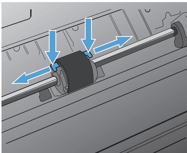
5. Gently pull the pickup roller up and out.
