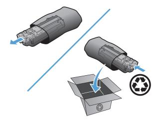
Grasp both sides of the print cartridge and gently rock the print cartridge to distribute the toner evenly inside the cartridge.
