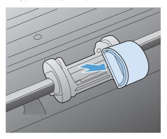
Position the new pickup roller in the slot. The circular and rectangular slots on each side prevents you from installing the roller incorrectly.
