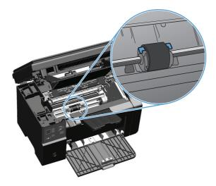
Release the small, white tabs on each side of the pickup roller, and rotate the pickup roller toward the front.
