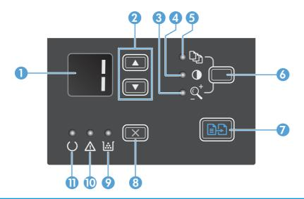
**LED display screen**: Displays the number of copies, the level of darkness for copies, and the percentage of copy-size reduction or enlargement. It also shows error codes that alert you of problems that require attention.
