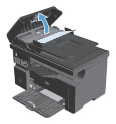
Carefully remove jammed paper. Gently try to remove the page without tearing it.
