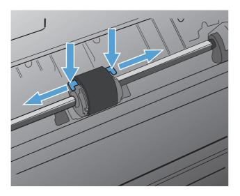
Gently pull the pickup roller up and out.
