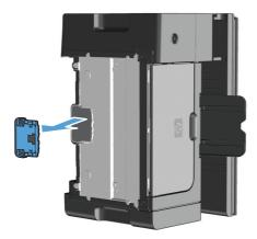
5. Dab a lint-free cloth in isopropyl alcohol, and scrub the separation pad. Use a dry, lint-free cloth to remove the loosened dirt, and wait for the separation pad to dry.
