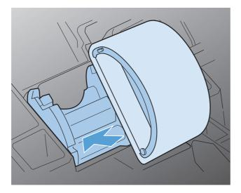
Rotate the top of the new pickup roller away from you until both sides snap into place. **7.**
