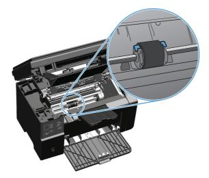
**4.** Release the small, white tabs on each side of the pickup roller, and rotate the pickup roller toward the front.
