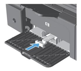
When finished printing with short media, remove the short media extender tool, and then place it back in the storage slot.
