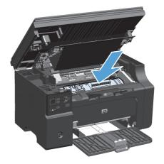
Close the print-cartridge door and the scanner assembly.
