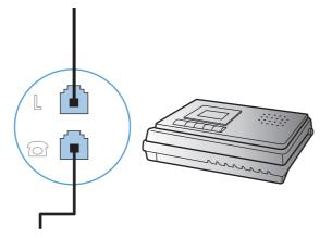
7. To connect a telephone, plug a telephone cord into the previous device's "telephone" port. Plug the other end of the telephone cord into the telephone "line" port.
