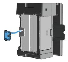
Insert the new separation pad, and screw it into place.
