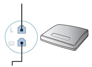
6. To connect an answering machine, plug a telephone cord into the previous device's "telephone" port. Plug the other end of the telephone cord into the answering machine "line" port.
