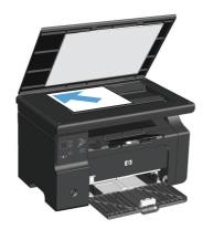
2. Press the Setup 🔲 button, and make sure that the Number of Copies 🕒 light is on.
