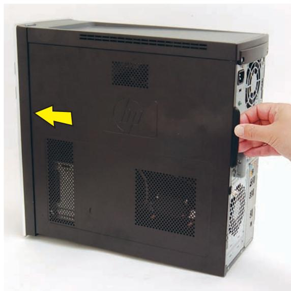
**16** Tighten the side panel thumbscrew on the back of the computer.
