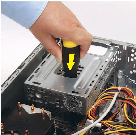
**14** Using the screwdriver, press the latch for the drive cage inside the computer.
