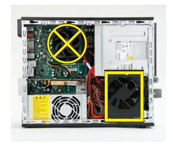
Remove the system fan screw. (This is one of the short screws on select models.)
