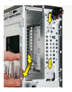
**20** Lift the cage all the way out of the computer and set it on its side.
