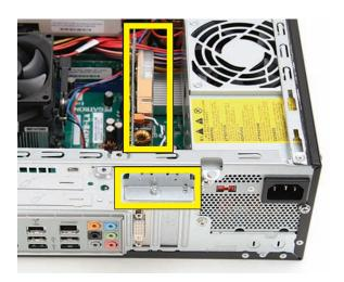
**8** Remove the screw from the bracket cover for the add-in cards.
