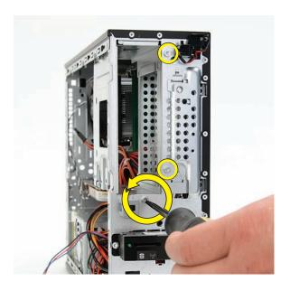
Remove the drive cage by moving it downward to release it, and then lifting it partway out of the computer.
