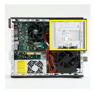
**9** Locate the cables connected to the back of the drive. Your drive may have three or two cables.
