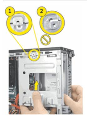
**7** Replace the screw at the top of the drive cage.
