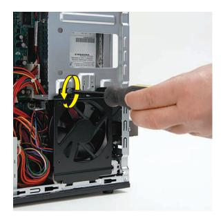
Push in the metal tab (1) above the fan as you tip out the top of the fan (2), and lift the fan (3) partway out of the computer. Without disconnecting the fan, set it aside.
