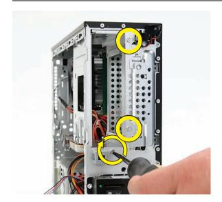
9 Replace the system fan by inserting the two lower hooks on the fan (1) into the slots in the computer, and then swinging the top of the fan (2) onto the computer.
