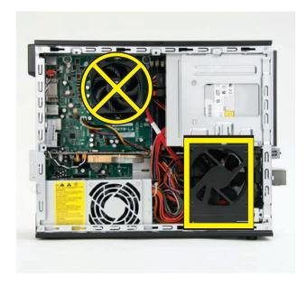
**9** Remove the system fan screw.
