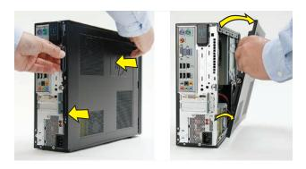
**6** Locate the three tabs that secure the front panel to the computer. Pull each of the tabs out slightly, away from the computer, to release the panel.
