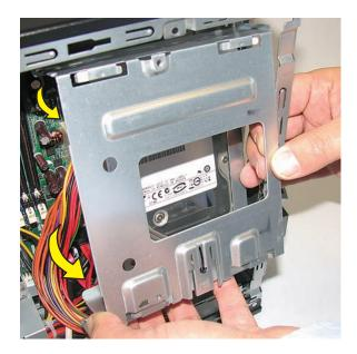
21 Locate the cables connected to the hard disk drive.
