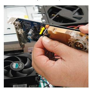
2 Align the edge of the add-in card with the open slot (1) in the computer, and then press the card straight down until it is fully seated in the socket (2).
