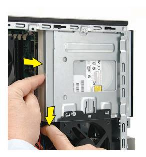
Pull the drive completely out the front of the computer, and then set it aside.
