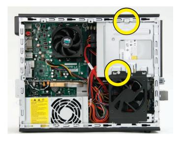
Below are the locations of the three long screws (select models) for the drive cage on the front of the computer.
