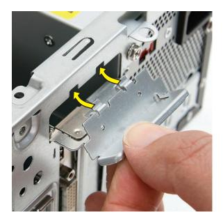
4 Insert and tighten the bracket cover screw.
