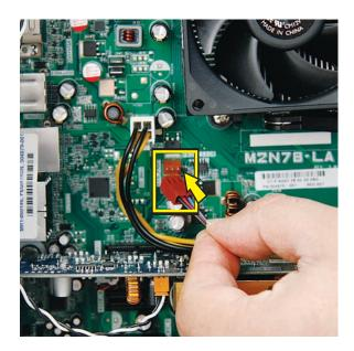
2 Replace the system fan by inserting the two lower hooks on the fan (1) into the slots in the computer, and then swinging the top of the fan (2) onto the computer.
