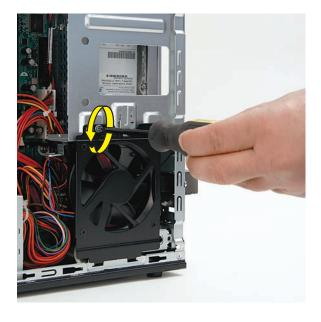
**10** Push in the metal tab (1) above the fan as you tip out the top of the fan (2), and lift the fan (3) partway out of the computer.
