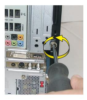
5 Slide the side cover toward the back of the computer, lift it off, and set it aside.
