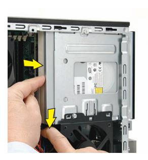
**13** Pull the drive completely out the front of the computer, and then set it aside.
