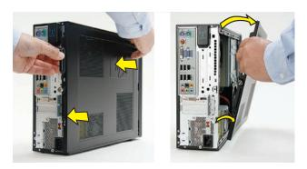
Locate the three tabs that secure the front panel to the computer. Pull each of the tabs out slightly, away from the computer, to release the panel.
