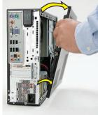
Locate the three tabs that secure the front panel to the computer. Pull each of the tabs out slightly, away from the computer, to release the panel.
