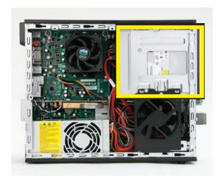
**9** Locate the cables connected to the back of the drive. Your drive may have three or two cables.
