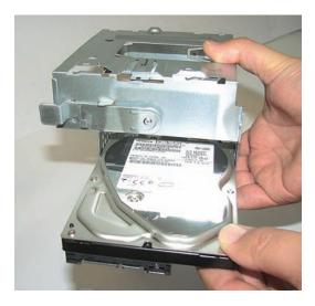
2 Slide the drive into the drive cage, and align the four screw holes in the sides of the drive with the holes in the cage.
