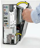
Locate the three tabs that secure the front panel to the computer. Pull each of the tabs out slightly, away from the computer, to release the panel.
