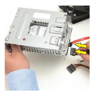
5 Tip the drive cage and insert it into the computer.
