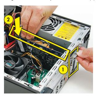
**3** Align the tabs on the bracket cover with the slots on the back of the computer and replace the bracket cover.
