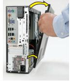
**6** Locate the three tabs that secure the front panel to the computer. Pull each of the tabs out slightly, away from the computer, to release the panel.
