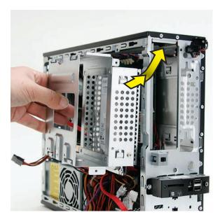
**6** Align the drive cage with the opening in the front of the computer, slide the drive cage up to engage the two tabs, circled below, and...
