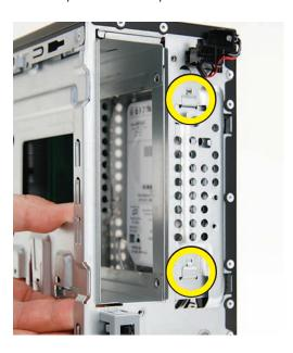
...ensure the screw hole at the top of the drive cage aligns under the screw hole in the computer rail (1).
