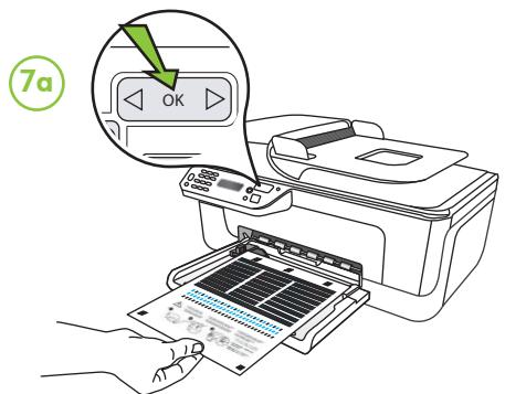
**EN** Align the print cartridges
