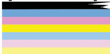
**Figure 11-3 Color bars - color mixing (yellow bar contains magenta streaks)**
