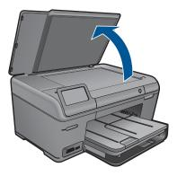
Load original print side down on right front corner of glass.
