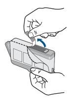
**b**. Twist orange cap to snap it off. A forceful twist may be required to remove cap.
