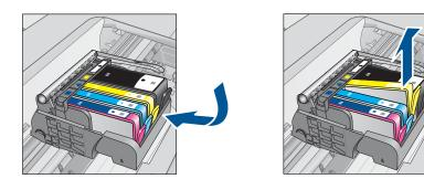
4. Lift the latch handle on the print carriage until it stops.
