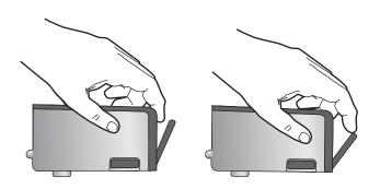
**11.** Reinstall the ink cartridge. It should now snap down into place.
