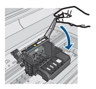
**Cause:** The print carriage latch was not closed properly. If this did not solve the issue, try the next solution.
