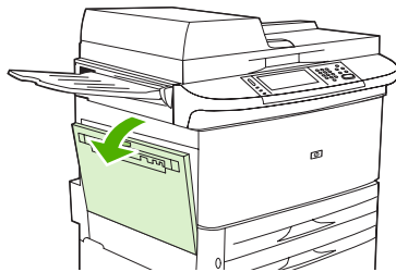
Figure 12-3 Clear jams in the duplex printing accessory (2 of 6)
