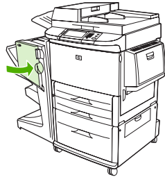
Figure 12-51 Clear a staple jam from the multifunction finisher (11 of 11)
