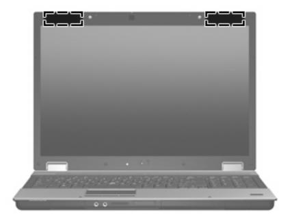
NOTE: For optimal transmission, keep the areas immediately around the antennas free from obstructions.
