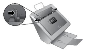
When scanning small originals such as checks, it is especially important that the paper guides fit snugly against the edges of the original.
