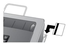
Use the card slot of the back of the scanner to scan rigid items such as laminated cards and embossed cards. The card slot accepts cards with raised characters. (Use the document feeder to scan flexible items such as business cards.)
