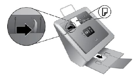
2. Adjust the paper guides to center the original. Make sure the paper guides touch the edges of the original.
