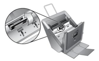
Clean the glass by using a soft, lint-free cloth that has been sprayed with a mild glass cleaner.
