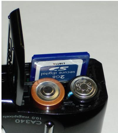
**Figure 1 SD card slot on HP CA340 Digital Camera**
