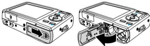
3. Insert the batteries into the compartment with the terminal facing inside the camera and the batteries indent next to the compartment door.
