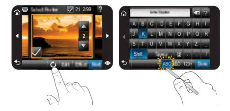
Use your fingers on the touch screen for most operations, such as menu navigation or selecting options in the touch screen frame. For more information, see The touch screen frame. The printer chirps once for each button press. You can change the volume of the sounds or turn them off in the Preferences menu. You can also use the stylus for these activities, but it is designed primarily for drawing and entering captions through the touch screen keyboard. For more information, see Use the stylus.
