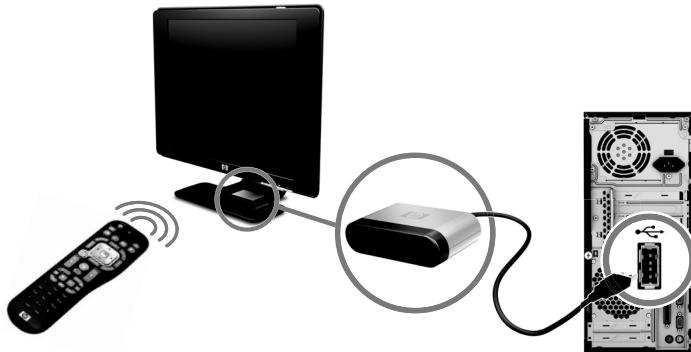
To use the remote control, point it in a direct line of sight at the remote sensor. The remote control and the sensor can be no farther than 8 meters (26 feet) apart. The remote control can be no more than 22.5 degrees (45 degrees total) from the center of the remote sensor.
