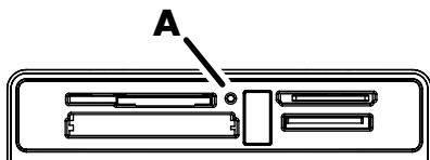
The activity light (**A**) blinks to indicate that the computer is accessing the memory card to read or write.
