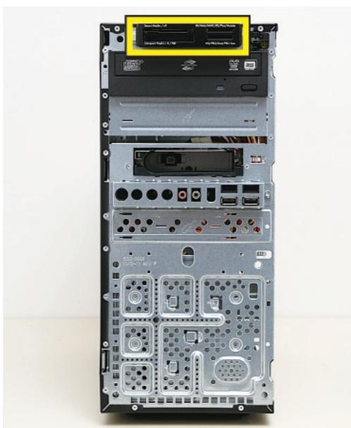
**10** Remove the screw that secures the reader in the computer.
