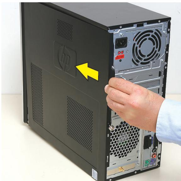
**15** Tighten the side panel thumbscrew on the back of the computer.
