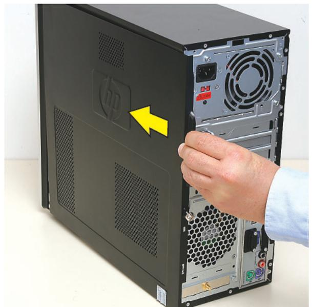
8 Tighten the side panel thumbscrew on the back of the computer.
