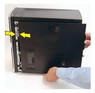
**3** Place the bottom of the panel on the computer, inserting the tabs on the inside of the panel into the rail slots on the computer. Swing the top of the panel toward the computer, inserting the top tabs into the rail slots.
