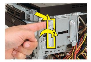
**4** Push the drive completely into the computer, until the optical drive latch locks it into place in the hole labeled 2 on the computer.
