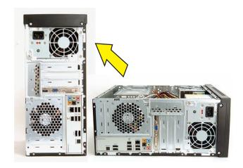
11 Hold the front panel over the computer, and then press the left side of the panel, inserting the tabs into the computer. Swing the right side of the panel toward the computer, and then press it into the computer.
