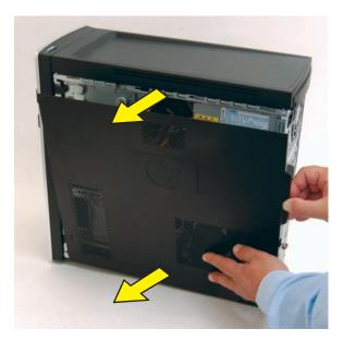
7 Locate the three tabs that secure the front panel to the computer. Pull each of the tabs out slightly, away from the computer, to release the panel.
