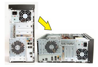
**10** Locate the hard disk drive cage inside the computer. You must remove the cage to access memory.
