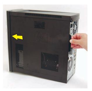
**5** Tighten the side panel thumbscrew on the back of the computer.
