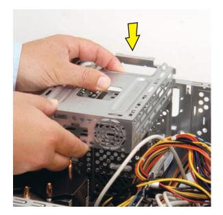
7 Slide the cage toward the bottom of the computer until it locks into place.
