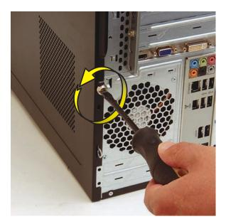
5 Grasp the handle, and pull the side panel about 2.5 cm (1 inch) toward the back of the computer to release it.
