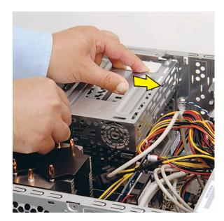
**16** Lift the cage partway out of the computer.
