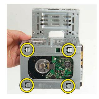
**5** Locate the four slots inside the computer that match the tabs on the bottom of the hard disk drive cage.
