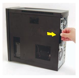
**6** Tilt out the top of the side panel, and then lift the panel from the computer.
