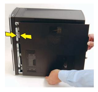
Place the bottom of the panel on the computer, inserting the tabs on the inside of the panel into the rail slots on the computer. Swing the top of the panel toward the computer, inserting the top tabs into the rail slots.
