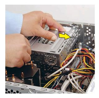
Lift the cage partway out of the computer.
