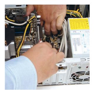
• If there is no release latch, rock the card to free it, and then lift the card from the socket.
