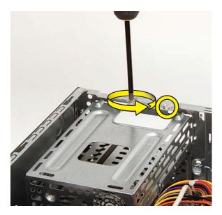
Insert a long screwdriver into the opening in the cage.
