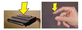
For plugs with a latch, press the latch (1 or 3) in the center of each plug, and then pull the plug (2 or 4) from the connector.
