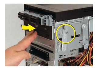
5 Hold the front panel over the computer, and then press the left side of the panel, inserting the tabs into the computer. Swing the right side of the panel toward the computer, and then press it into the computer.
