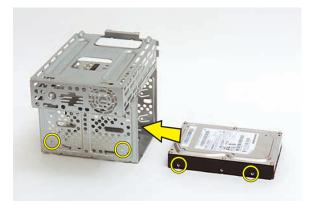
**2** Insert and tighten the four screws that secure the drive in the cage.
