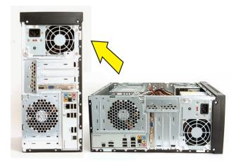
**12** Hold the front panel over the computer, and then press the left side of the panel, inserting the tabs into the computer. Swing the right side of the panel toward the computer, and then press it into the computer.
