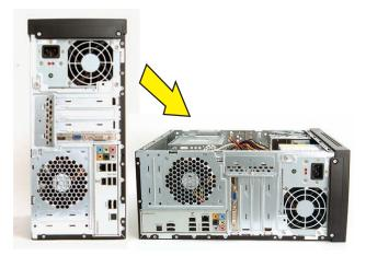
Remove the two screws that secure the drive cage in the computer.
