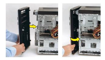
6 Hold the side panel over the side of the computer with the front edge of the panel about 2.5 cm (1 inch) from the front of the computer.
