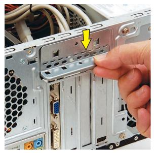
**5** Insert and tighten the bracket cover screw. If it is present, also insert and tighten the additional screw that secures a large graphics card.
