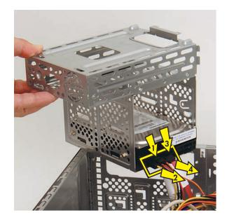
**18** Remove the four screws (two on each side) that secure the drive in the cage.
