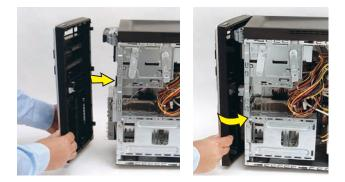
2 Hold the side panel over the side of the computer with the front edge of the panel about 2.5 cm (1 inch) from the front of the computer.
