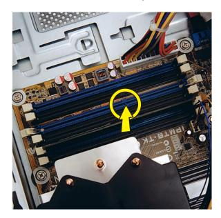
**3** Position the memory module over the socket, aligning the notch with the tab in the socket, and then firmly press the module down into the socket...
