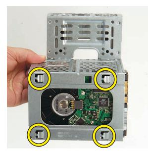
**4** Locate the four slots inside the computer that match the tabs on the bottom of the hard disk drive cage.
