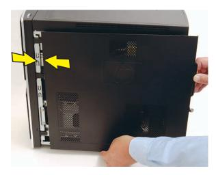
7 Place the bottom of the panel on the computer, inserting the tabs on the inside of the panel into the rail slots on the computer. Swing the top of the panel toward the computer, inserting the top tabs into the rail slots.
