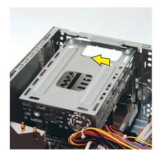
**9** Insert and tighten the two screws that secure the cage in the computer.
