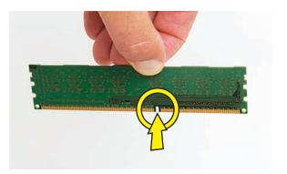
**2** Look at the memory module socket for the tab that matches the notch on the memory module.
