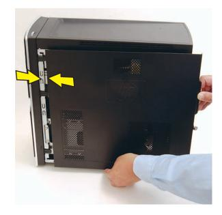
8 Place the bottom of the panel on the computer, inserting the tabs on the inside of the panel into the rail slots on the computer. Swing the top of the panel toward the computer, inserting the top tabs into the rail slots.
