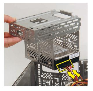
7 Lower the cage into the computer, inserting the four tabs on the bottom of the cage into the computer slots.
