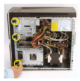
**9** Swing the front panel open toward the left, and then lift it off the computer.
