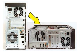
8 Locate the add-in cards on the back of the computer. Identify the one you want to replace.
