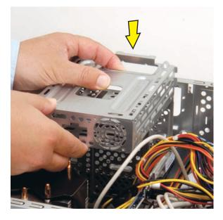
8 Slide the cage toward the bottom of the computer until it locks into place.
