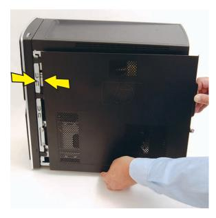
14 Place the bottom of the panel on the computer, inserting the tabs on the inside of the panel into the rail slots on the computer. Swing the top of the panel toward the computer, inserting the top tabs into the rail slots.
