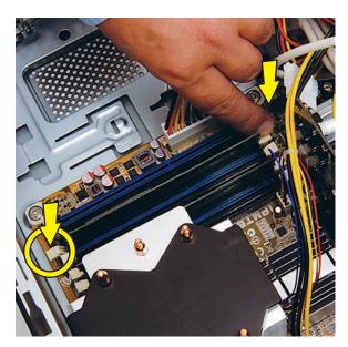
**20** Touching only the top edge of the memory module, lift it out of the socket.
