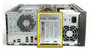
On the back of the computer, remove the screw from the bracket cover for the add-in cards. If it is present, also remove the additional screw that secures a large graphics card.
