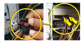
**3** Pull out the optical drive latch (1), swing it to the right (2), and release it into the hole labeled 2 on the computer.
