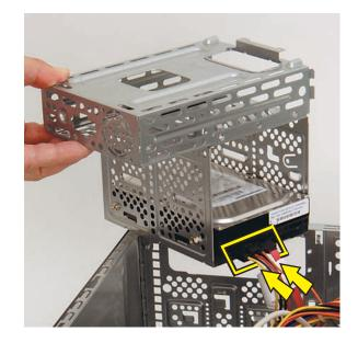
**6** Lower the cage into the computer, inserting the four tabs on the bottom of the cage into the computer slots.
