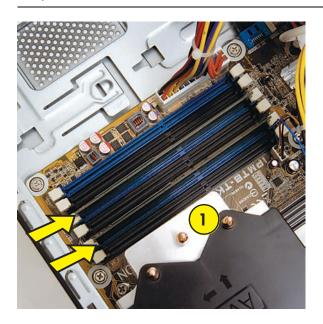
**19** Push down the retaining clip on each end of the memory socket to release the memory module.
