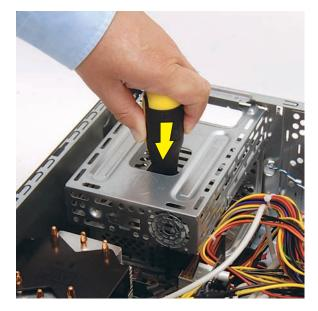
Using the screwdriver, press the latch for the drive cage inside the computer.
