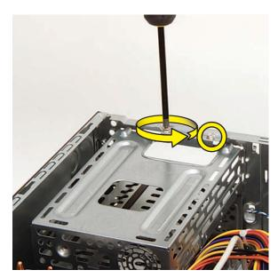
Insert a long screwdriver into the opening in the cage.
