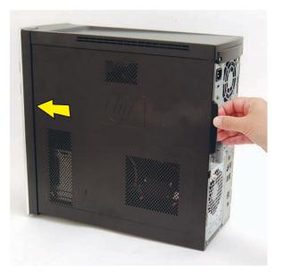
**10** Tighten the side panel thumbscrew on the back of the computer.
