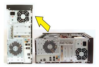
7 Hold the side panel over the side of the computer with the front edge of the panel about 2.5 cm (1 inch) from the front of the computer.
