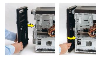
**13** Hold the side panel over the side of the computer with the front edge of the panel about 2.5 cm (1 inch) from the front of the computer.
