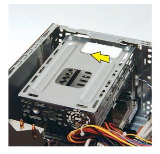
8 Insert and tighten the two screws that secure the cage in the computer.
