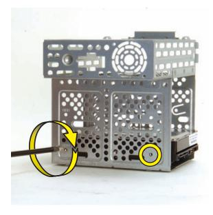
**3** Tip up the hard disk drive cage, and locate the four tabs on the bottom.
