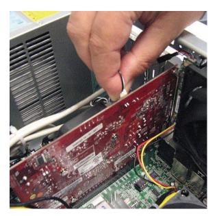
**3** Look at the bracket cover for the two hooks that fit over the two slots on the back of the computer.
