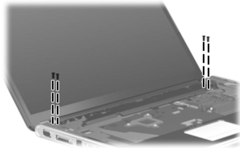
**Where used:** 4 screws that secure the display assembly to the computer
