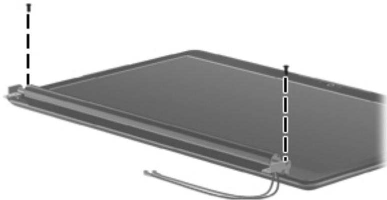
**Where used:** 2 screws that secure the display bezel to the display
