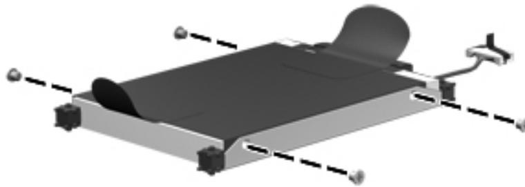
**Where used:** 4 screws that secure the hard drive bracket to the hard drive
