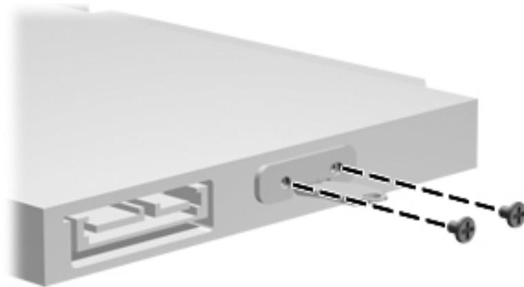
**Where used:** 2 screws that secure the optical drive bracket to the computer.
