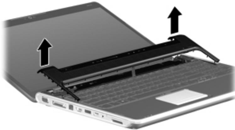
5. Move the switch cover back so that it rests on the display.
