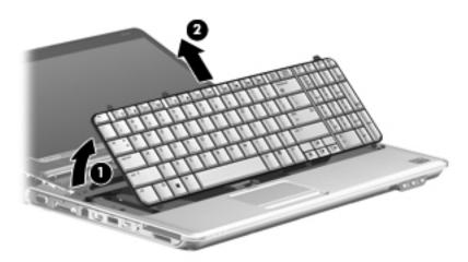
9. Release the zero insertion force (ZIF) connector **1** to which the keyboard cable is connected and disconnect the cable **2** from the system board.
