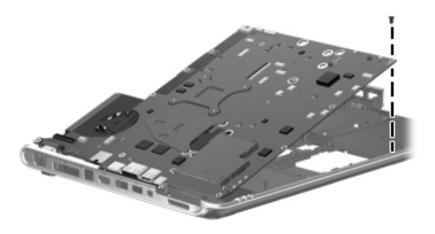
Where used: One screw that secures the system board to the base enclosure
