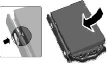
2. Flex the front of the right side rail and insert the pin into the hard drive's mounting hole, and then flex the back of the right side rail and insert the pin into the other mounting hole.
