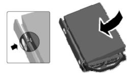
8. Flex the right side rail, and then insert the pins into the hard drive's mounting holes.
