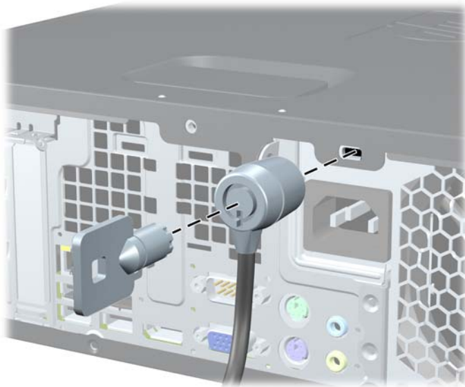
Figure C-1 Installing a Cable Lock
