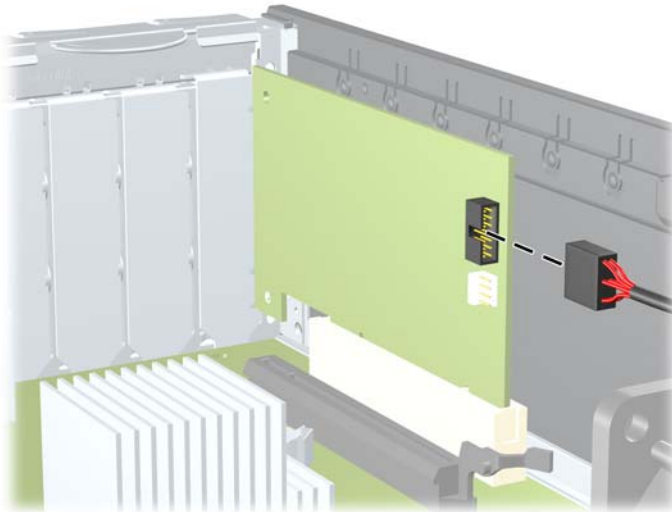
Figure 2-30 Disconnecting the Media Card Reader 1394 Cable
