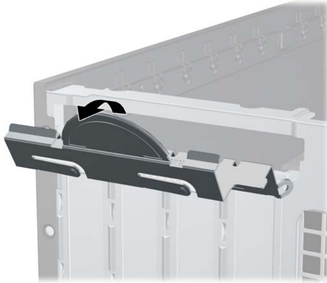
Figure 2-11 Opening the Expansion Slot Retainer
