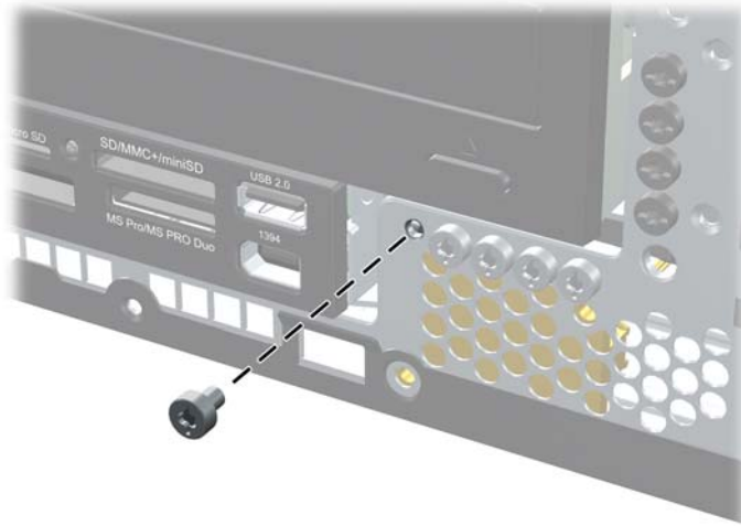
Figure C-7 Retrieving the Front Bezel Security Screw
