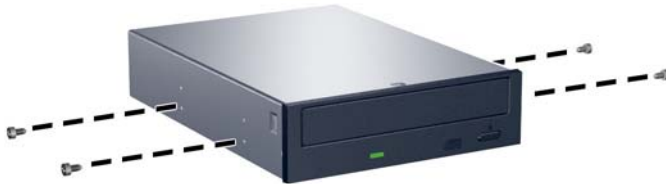
Figure 2-24 Installing Guide Screws in the Optical Drive
