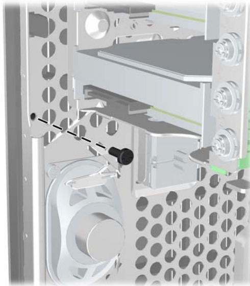
Figure C-8 Installing the Front Bezel Security Screw
