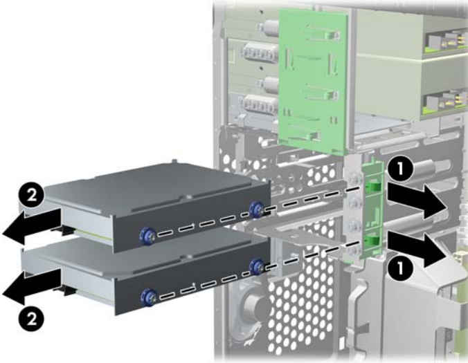
Figure 2-29 Removing a Hard Drive
