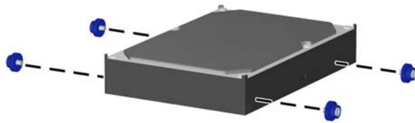
Figure 2-30 Installing Hard Drive Guide Screws
