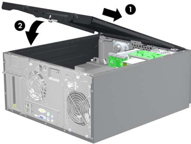
Figure 2-2 Replacing the Computer Access Panel
