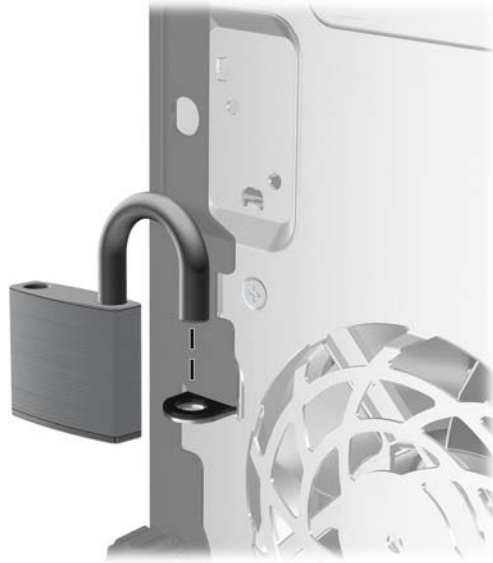
Figure C-2 Installation d'un cadenas
