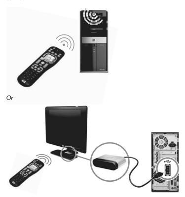
To use the remote control, point it in a direct line of sight at the remote sensor. The remote control and the sensor can be no farther than 8 meters (26 feet) apart. The remote control can be no more than 22.5 degrees (45 degrees total) from the center of the remote sensor.
