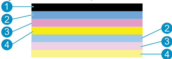
Figure 10-1 Color bars - expected result
