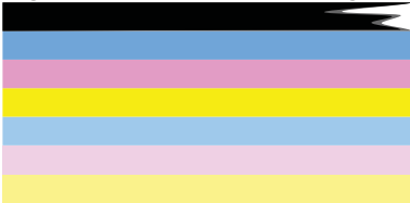
Figure 10-2 Color bars - irregularly streaked or faded bar (top bar)
