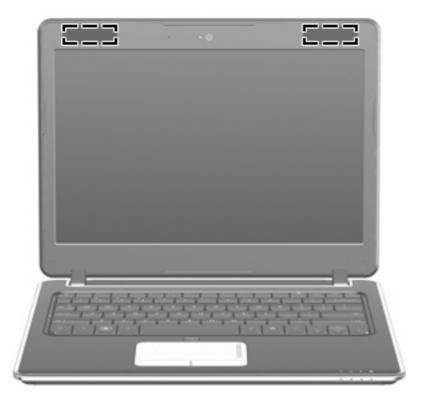
NOTE: For optimal transmission, keep the areas immediately around the antennas free from obstructions.
