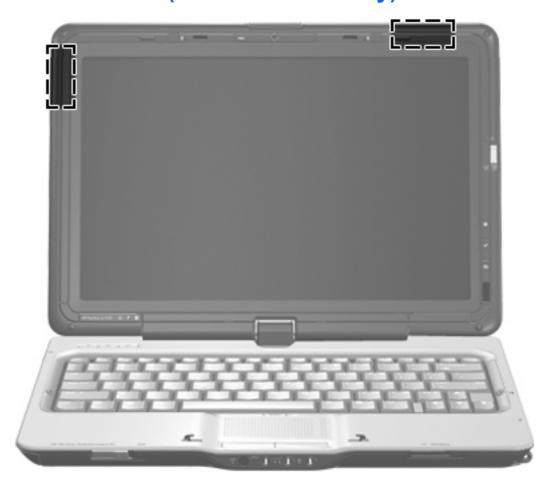
NOTE: For optimal transmission, keep the areas immediately around the antennas free from obstructions.
