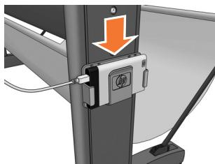
3. Connect the USB cable to the external hard disk.
