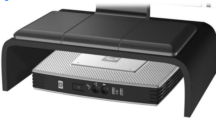
Figure D-3 Under monitor stand
