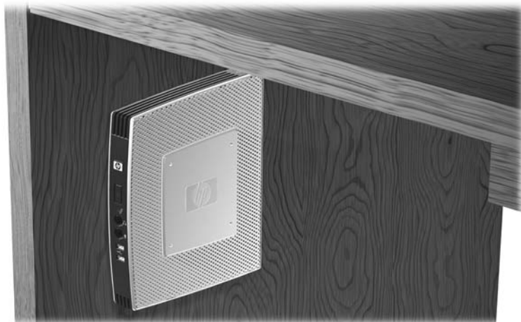
Figure C-8 Thin client mounted under desk
