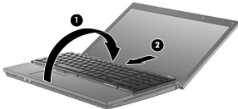
For 14-inch computers, turn over the keyboard (1) into the keyboard tray, and then slide the keyboard into place (2).
