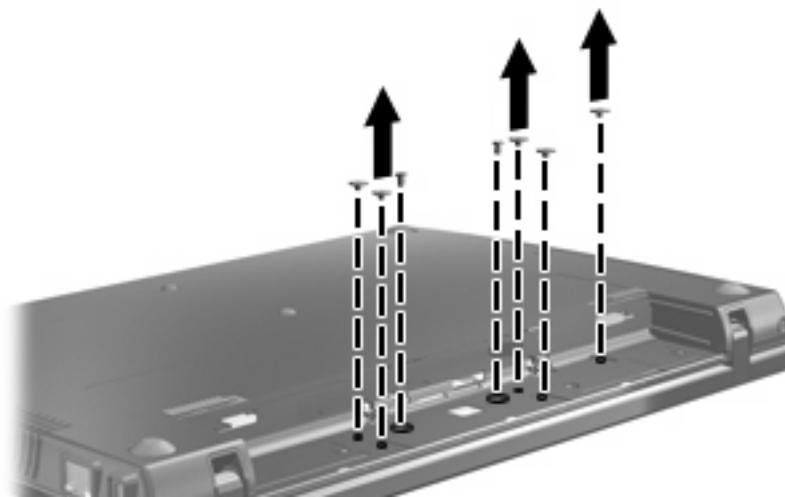
8. Turn the computer display-side up, and then remove the 2 screw covers and screws from the back edge of the computer.
