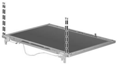
Where used: 4 screws that secure the display panel to the display enclosure
