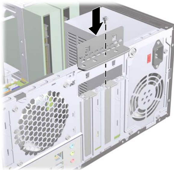
Figure 12 Securing the Expansion Cards and Slot Covers
