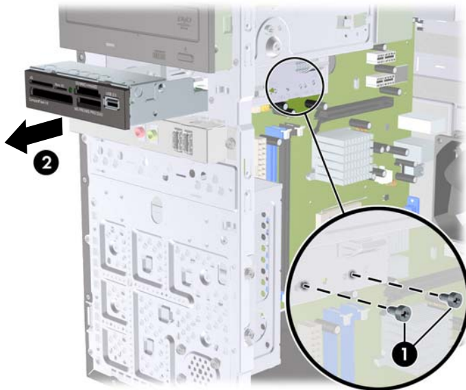
Figure 19 Removing a 3.5-inch Device (Media Card Reader Shown)
