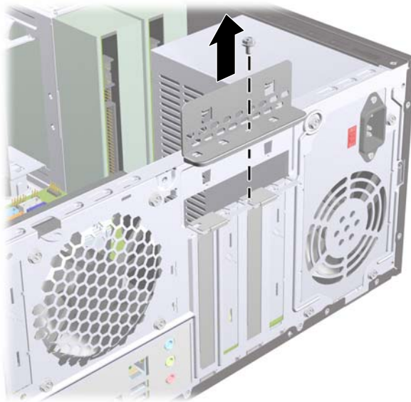
Figure 7 Opening the Slot Cover Lock
