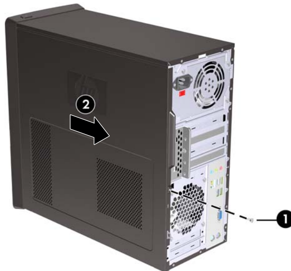
Figure 1 Removing the Computer Access Panel
