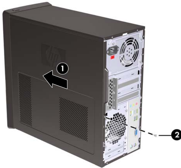
Figure 2 Replacing the Computer Access Panel
