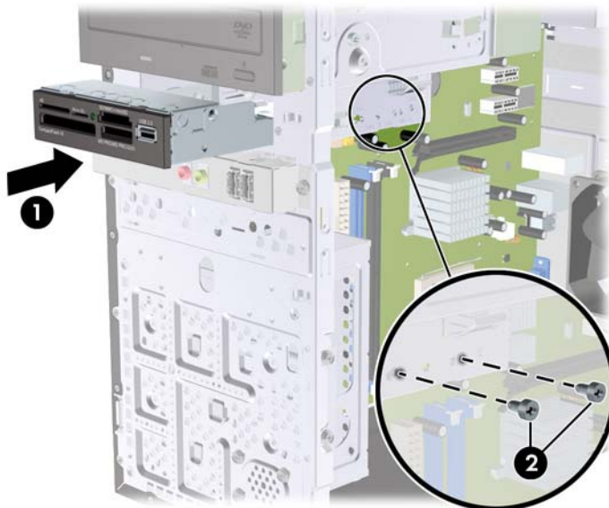
Figure 20 Installing a 3.5-inch Device (Media Card Reader Shown)
